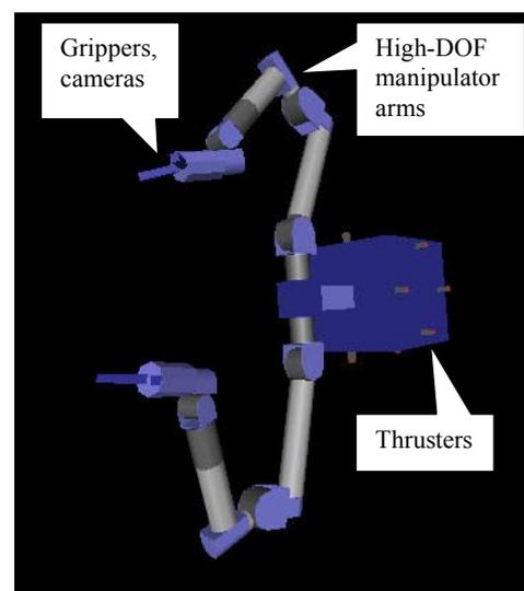
**Figure 1: Example robot concept for capture mission**
