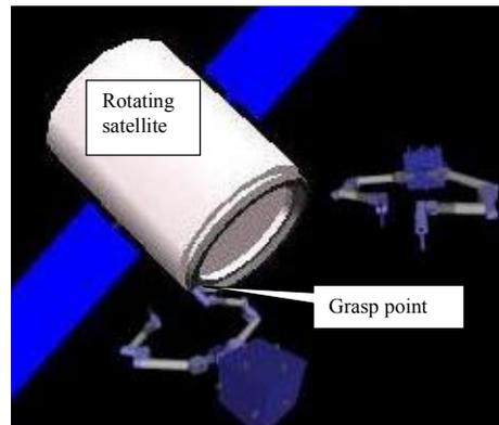
Figure 4: Robot grasps satellite on payload attachment fitting (PAF) Grasp, stabilization, and service.
