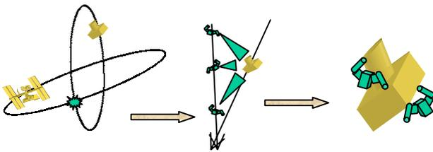
**Figure 6: Debris mitigation mission: potential collision, tracking, intercept, and disposal.**
