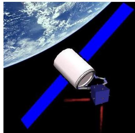
Figure 5: Robot uses its thrusters to stabilize the satellite's motion.
