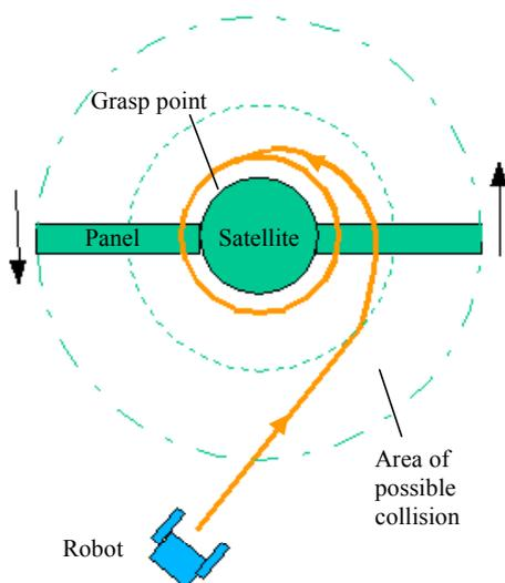
Figure 3. 2D Approach: robot approaches satellite in plane of panels and rotation.
