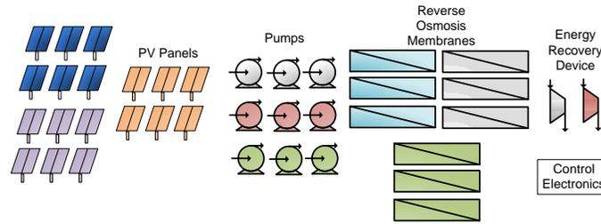
**Figure 3: Inventory used in modular design space analysis.**
