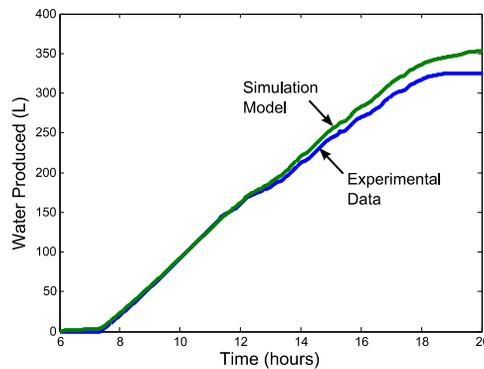
Figure 10: Experimental validation of modeling approach.
