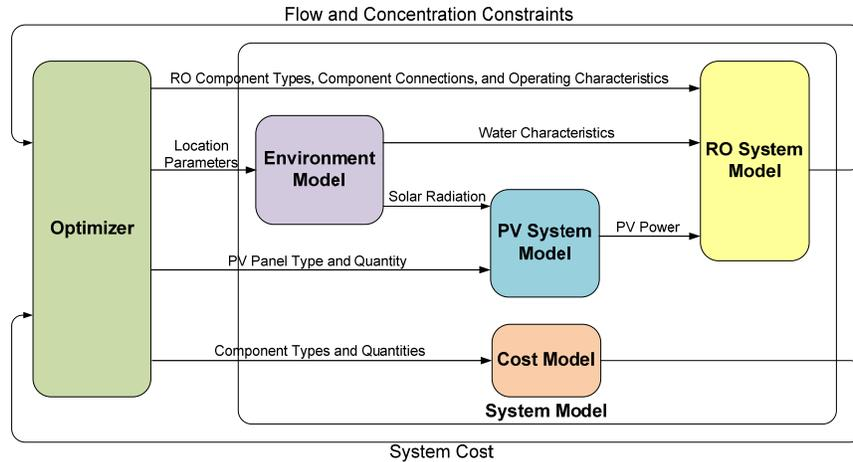
**Figure 4: Optimization and model setup.**
