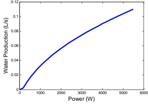
Figure 6: RO system water output for different power inputs.
