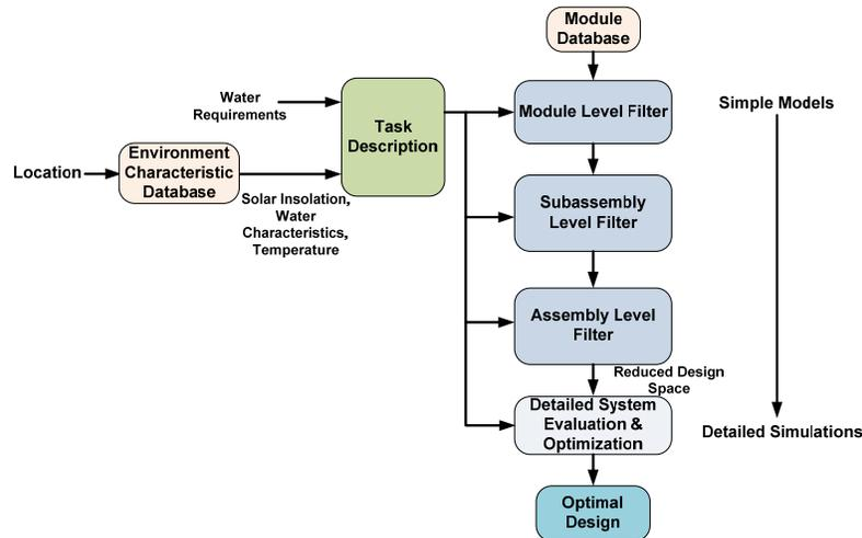
Figure 2: Modular design architecture.
