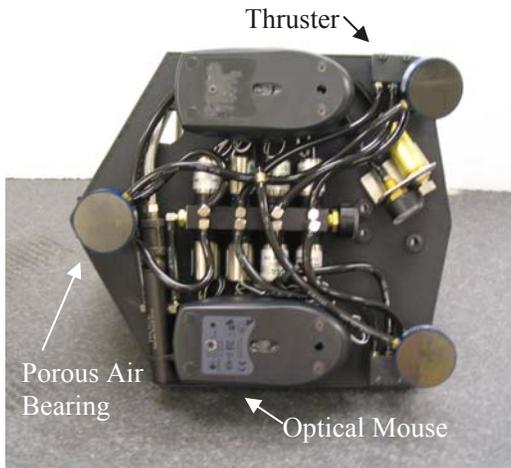
Fig. 15 (b) Bottom view of experimental space robot.
