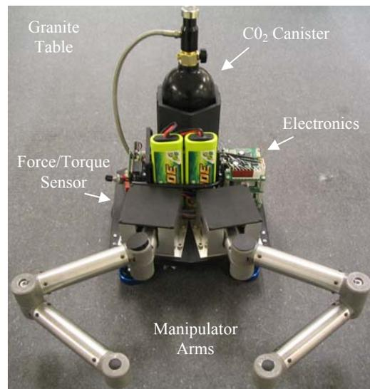
Fig. 15 (a) Front view of experimental space robot.
