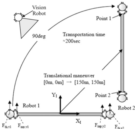
Fig. 6. Transportation maneuver using a team of robots.
