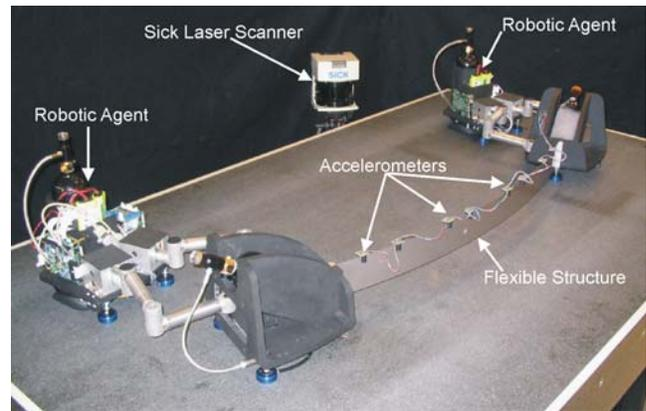
Fig. 14. Experimental system setup for sensor fusion experiments.
