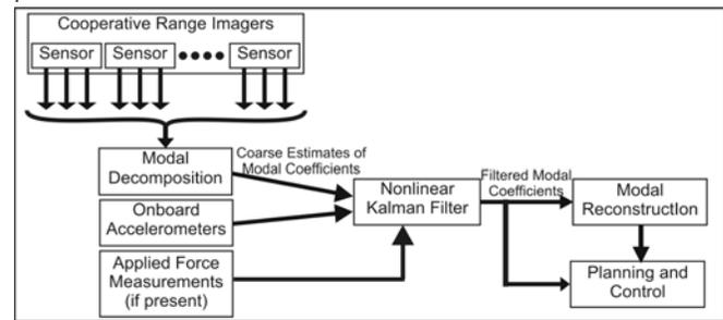
Fig. 5. FSE Estimation architecture
