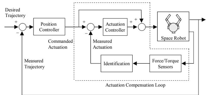
Fig. 4. Base Sensor Control (BSC). Inner loop identifies and compensates for actuator efforts while outer loop tracks desired trajectory
