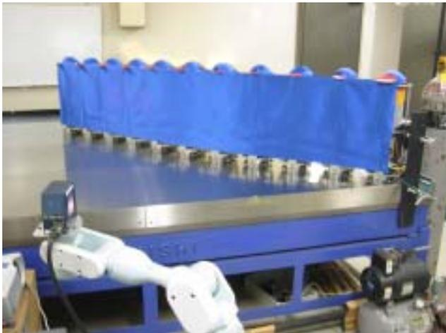
Fig. 9. Photograph of experimental system. Laser rangefinder mounted on manipulator arm can be seen in the foreground at left.
