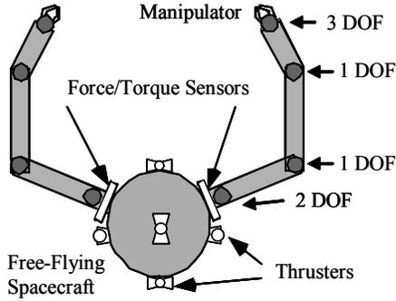
Figure 2. Space robot with force/torque sensors mounted between spacecraft and manipulator.
