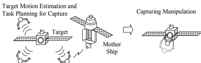
Figure 1. Mission scenario for robotic satellite capture
