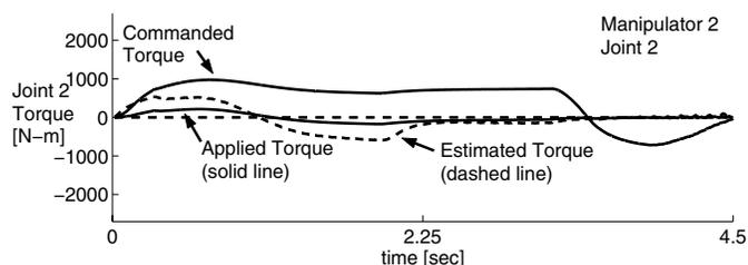
Figure 11. Manipulator 2 torques for the large satellite capture task
