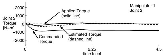
Figure 10. Manipulator 1 torques for the large satellite capture task
