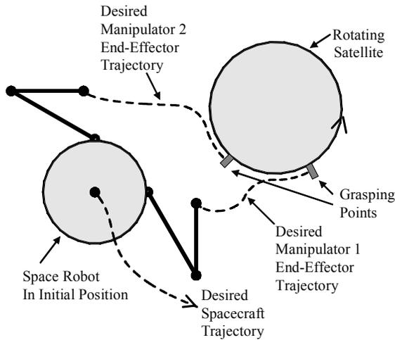
Figure 7. Desired spacecraft and manipulator end-effector trajectories
