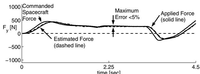
Figure 12. Continuous x and y commanded net thruster forces for the large satellite capture task
