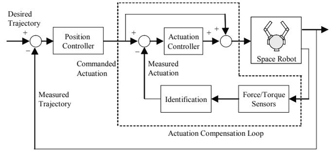
Figure 3. Inner loop identifies and compensates for actuator efforts while outer loop tracks desired trajectory.
