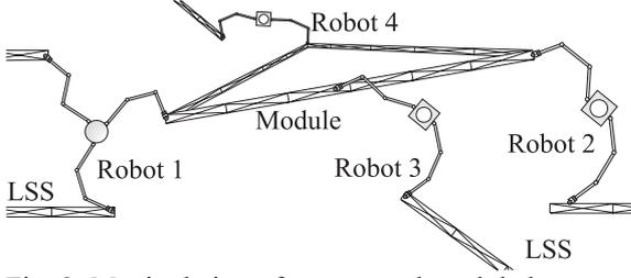
Fig. 2. Manipulation of a structural module by a team of multi-arm space robots.
