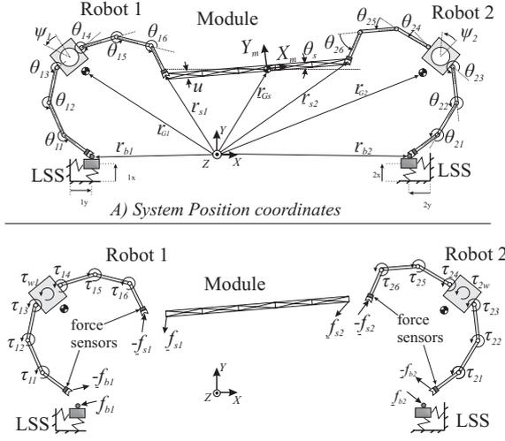
B) System Decomposition and System Force and Torque Elements
