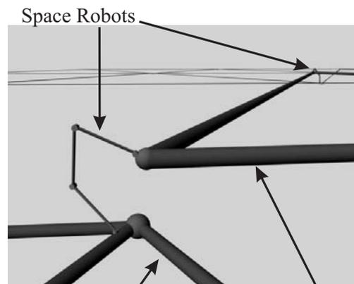
Fig. 1. Concept of using teams of robots to construct LSS by assembling large structural modules.
