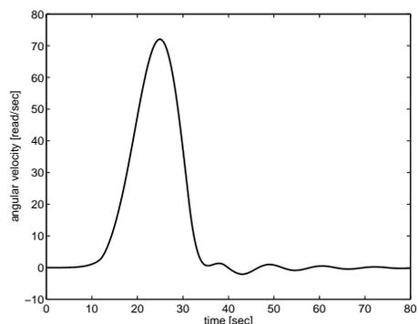
Fig. 11. Angular velocity of robot 1 reaction wheel.
