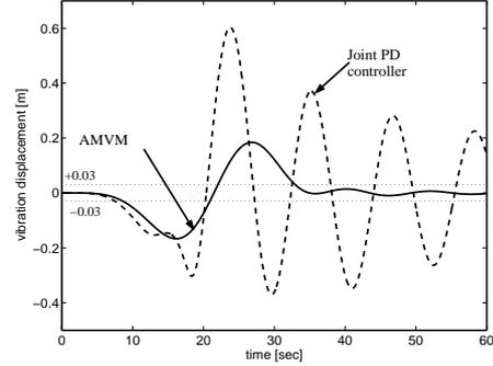
Fig. 6: Vibration displacement in the left beam end.
