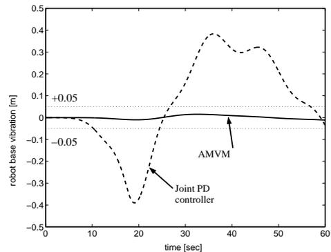
Fig. 8: Vibration displacement of the LSS in the grasping point of robot 1.
