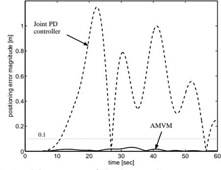
Fig. 5: Position error of the beam CM.
