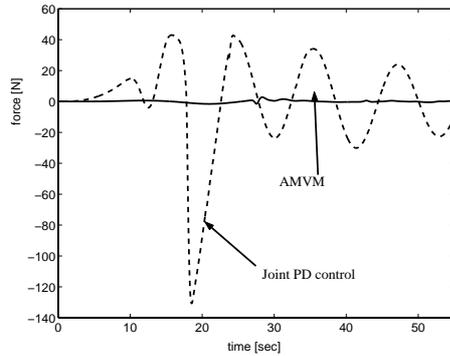
Fig. 7:  $Y$  component of the force that robot 1 applies to the LSS.
