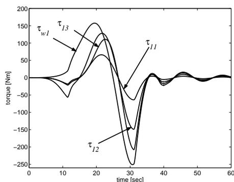
Fig. 10. Applied torque by the joint motors and by the reaction wheel motor of robot 1.
