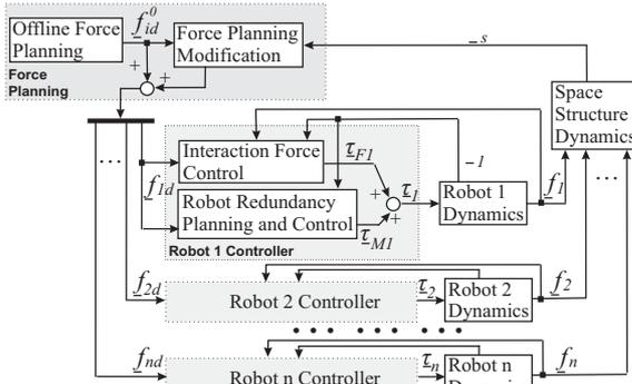
Fig. 3. Block diagram of the AMVM architecture.
