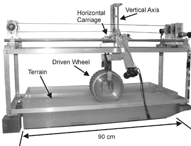
Fig. 4. FSRL wheel-terrain interaction testbed with FIDO wheel.
