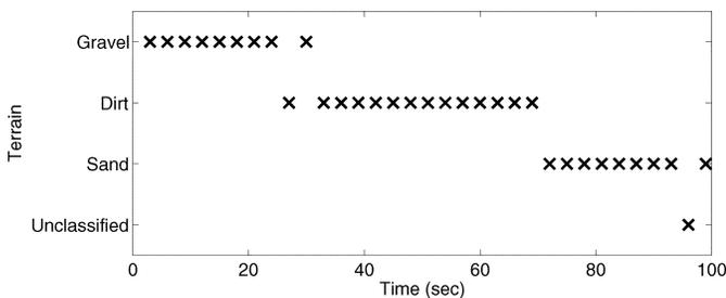
Fig. 10. Classification results for FSRL technology testbed rover traverse of gravel, packed dirt, and sand at 4 cm/s.
