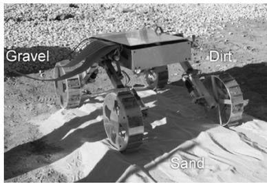
Fig. 7. FSRL technology testbed rover completing three-terrain traverse.
