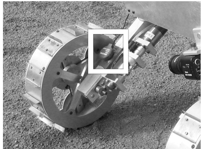
Fig. 8. Vibration sensor mounted on FSRL technology testbed rover.
