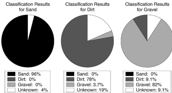
Fig. 9. Classification results for FSRL technology testbed rover vibration data.
