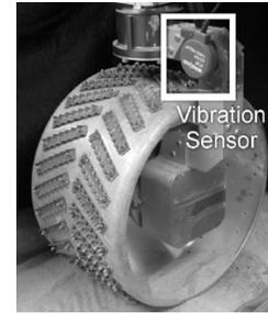
Fig. 5. Vibration sensor mounted on the FIDO wheel in the FSRL wheel-terrain interaction testbed.
