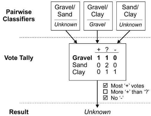
Fig. 3. Schematic of voting scheme resulting in unknown result.
