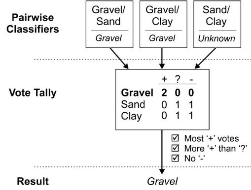
Fig. 2. Schematic of voting scheme positively identifying gravel.
