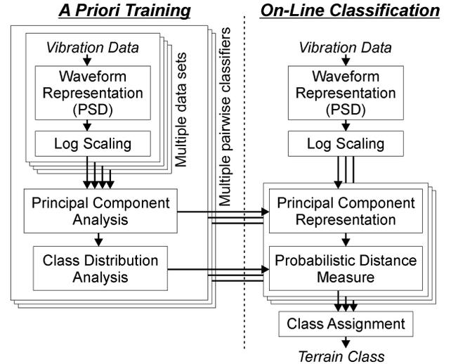
Fig. 1. Overview flowchart for vibration-based terrain-classification algorithm.
