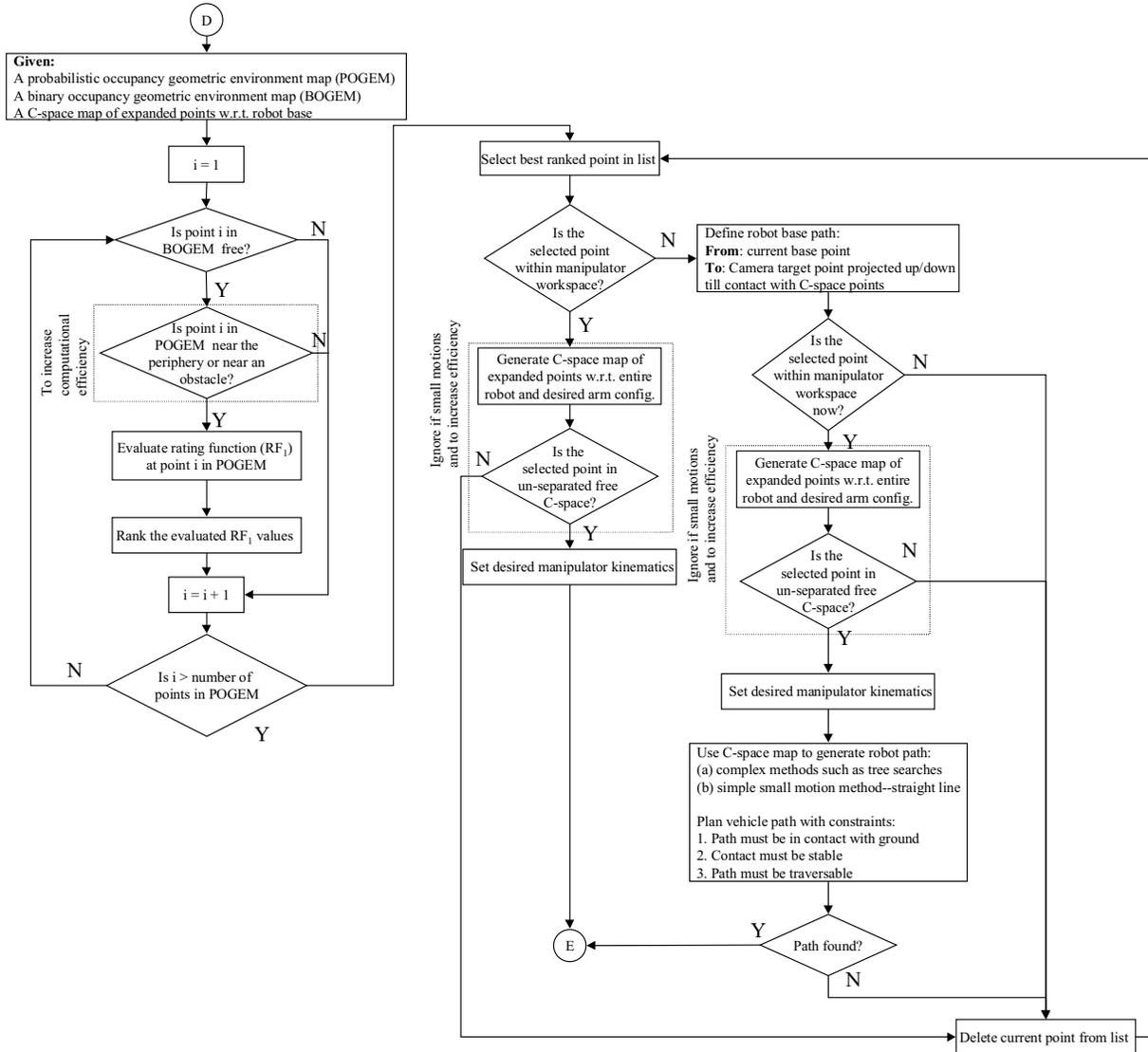
Fig. 7. Flowchart for vision system pose selection of environment mapping algorithm.
