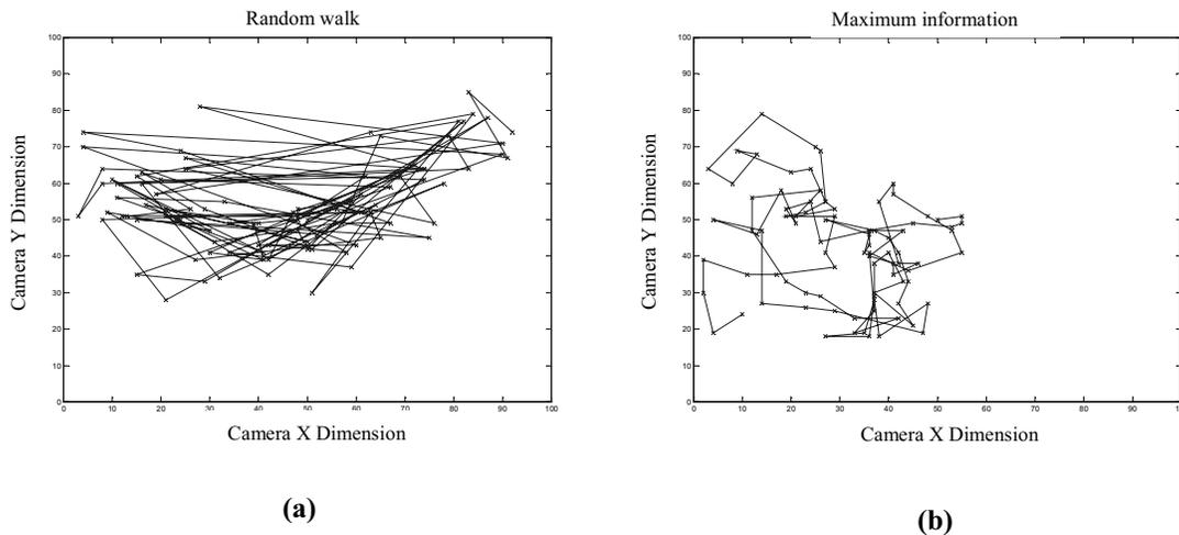
Fig. 14. Path taken by a single vision system: (a) random walk pose selection; (b) maximum information pose selection.
