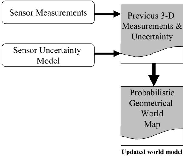
Fig. 4. 3D range measurement fusion with sensor uncertainty.
