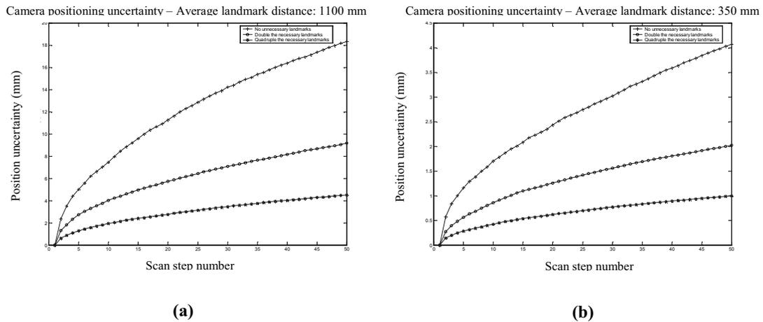
Fig. 15. Accumulated root-mean-square translation error of vision system: (a) average fiducial distance 1100 mm; (b) average fiducial distance 350 mm.
