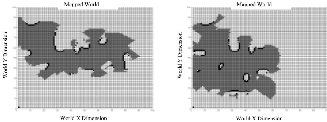
Fig. 13. Mapped area by a single vision system (gray = empty space; black = obstacle; white = unknown): (a) random walk pose selection; (b) maximum information pose selection.
