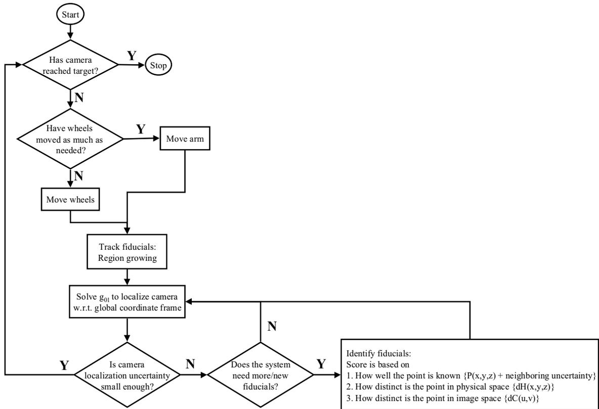
Fig. 9. Flowchart for vision system motion identification using scene fiducials.
