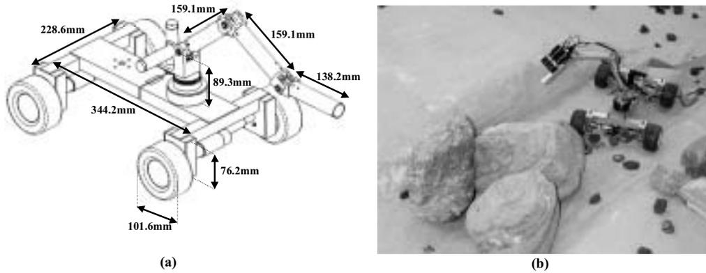
Fig. 16. Experimental mobile vision system modeling an unstructured environment: (a) schematic diagram of the physical system; (b) physical system implementation.
