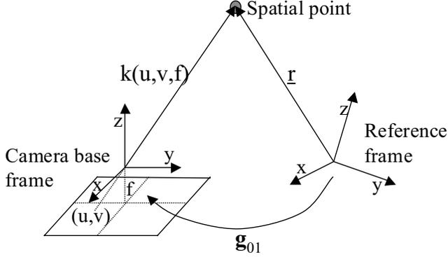
Fig. 8. Relationship of camera and target frames.
