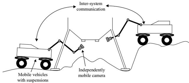
Fig. 2. Cooperative mapping by robots.
