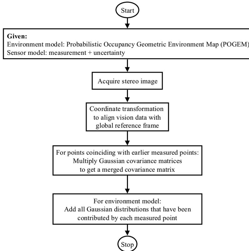
Fig. 5. Flowchart for data fusion using known vision system motion.
