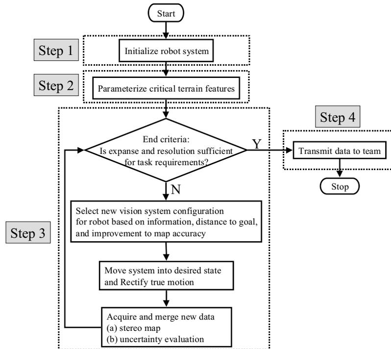
Fig. 3. Outline of model building and placement algorithm.
