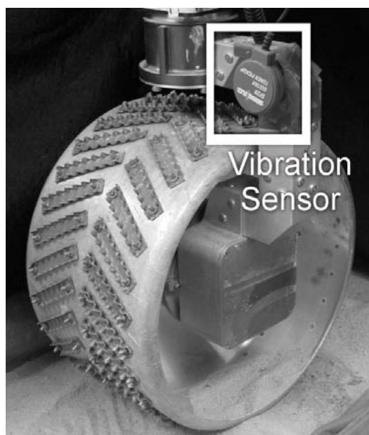
Fig. 9. Vibration sensor mounted on the FIDO wheel in the FSRL Wheel-Terrain Interaction Testbed
