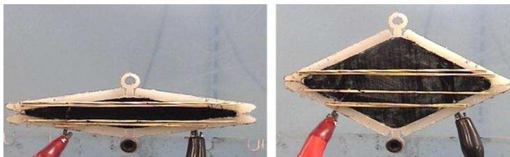
**FIGURE 9.** Experimental Dielectric Elastomer Actuator with 200 Percent Strain.
