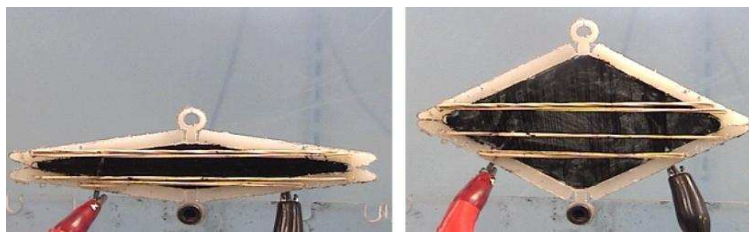
FIGURE 9. Experimental Dielectric Elastomer Actuator with 200 Percent Strain.
