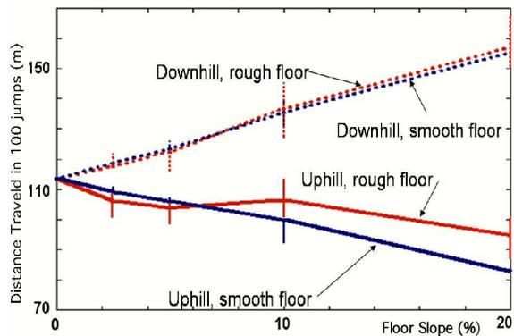
**FIGURE 7.** Variation of Microbot Range with Floor Slope
