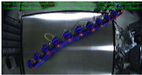
図2 CCD camera image of flexible structure (upper view)
