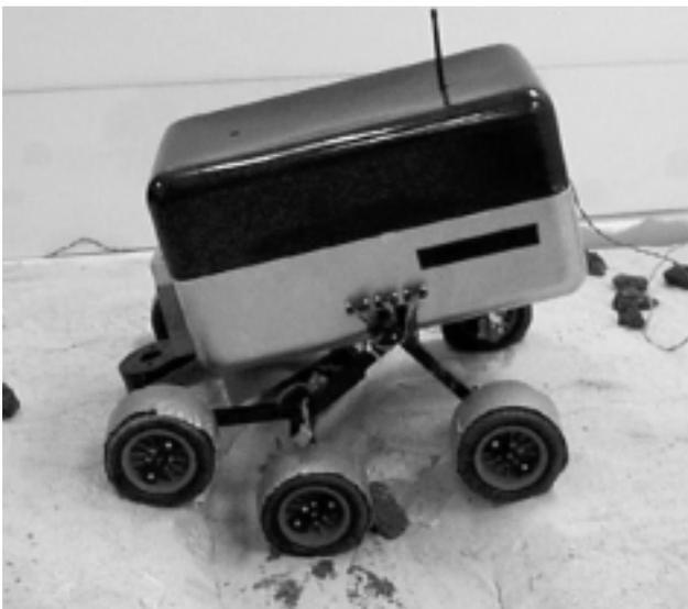
Fig. 15. Experimental microrover during go/no-go ditch traversal experiment.
