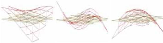
Fig. 3 Various Vibration Modes of a Typical Large Truss
