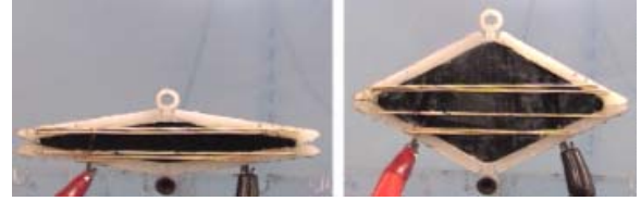
Figure 5. A Linear EPAM Actuator Shown in its ON (left) and OFF (right) Configurations
