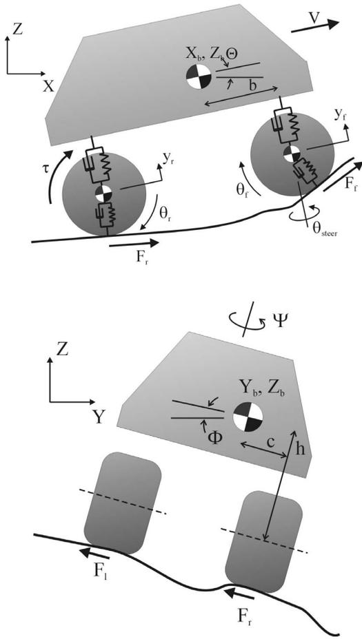
Figure 1. Schematic of high-speed mobile robot model.
