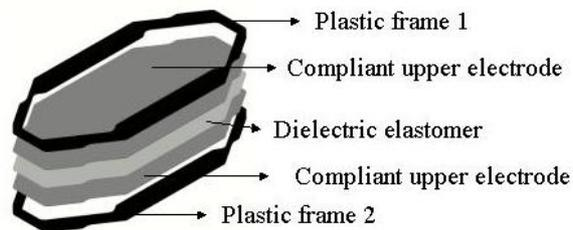
Fig.2. Exploded view of a linear polymer actuator. The compliant structures with leaf strings act as a restoring force to generate a two-way actuator.
