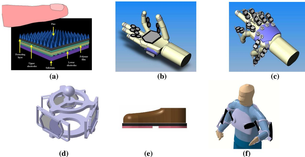
Fig.1. Applications of polymer actuators in virtual reality (a) tactile interface to generate different textures on the finger tip. (b) portable haptic interface mounted on the inner side of the hand (c) another haptic glove design on the finger phalanges (d) a fixed 3-dof haptic interface (e) Haptic shoe (f) Haptic interface to apply a force on the arms.
