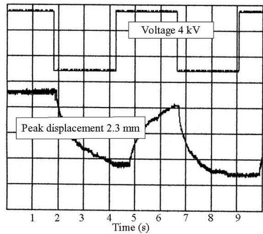
Fig. 10. Time response/ a square input of 0.25 Hz is applied
