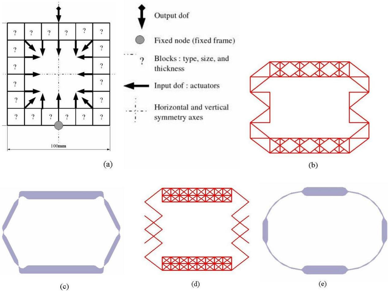
Fig.3. FlexIn: a new design method for compliant structures based on building blocks (a) Initial geometry with the boundary conditions. (b) solution 1 proposed by genetic algorithms. (c) Equivalent compliant structure for solution 1. (d) solution 2 proposed by genetic algorithms. (e) Equivalent compliant structure for solution 2.
