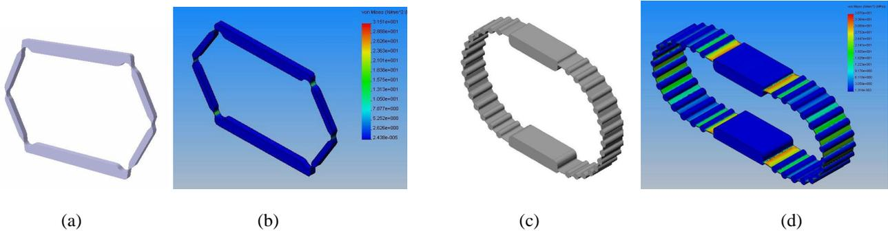
Fig.4. Different designs for the frame (a) Frame 1: notch flexure design (b) FEA (c) Frame 2: leaf spring design (d) FEA
