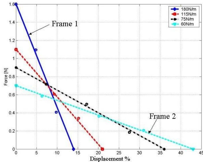
Fig.6. Force displacement curves of polymer actuators with frames of different stiffness.
