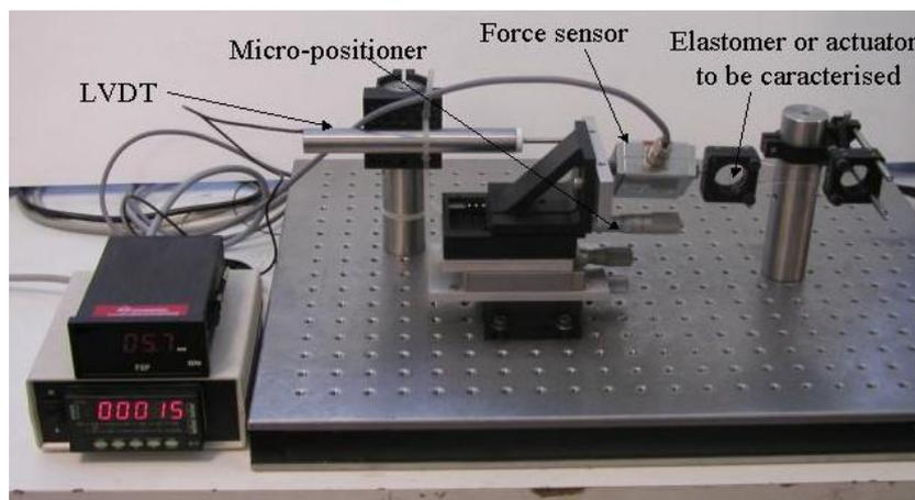
Fig.5. Experimental set-up to measure the force displacement curves of the different actuators design and to determine the stiffness of the active elastomer.
