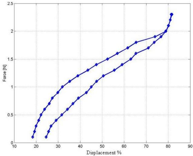
Fig. 7 stiffness of the 3M acrylic is determined. The polymer is stretched by 450% which generates plastic deformation.
