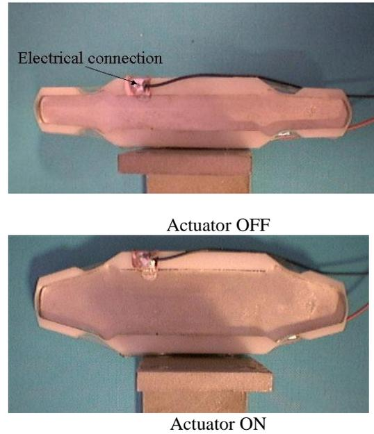
Fig. 8. The linear actuator presented has a compliant structure with leaf springs and is deformed by more than 40% when 4kV are applied.
