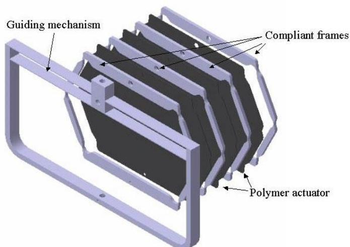
Fig.11. Improved actuator/ increasing the number of layer would increase the generated force.
