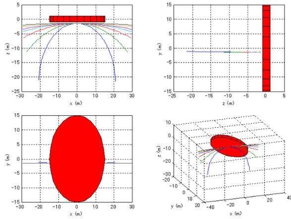
Fig.7 Relative position between approach trajectory and collision region (In-plane relative motion)
