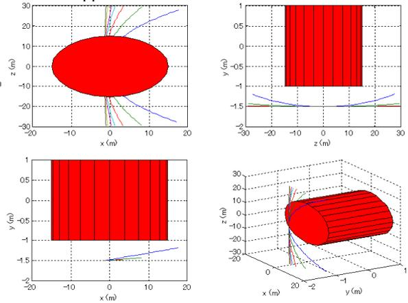
Fig.8 Relative position between approach trajectory and collision region (Out-of-plane relative motion)
