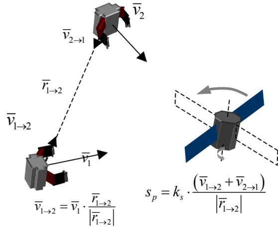
Fig. 9 Safety Metric Based on Relative Velocity and Distance
