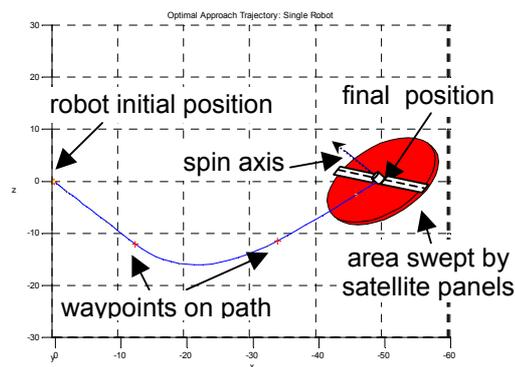
Fig. 10 Optimal Approach Trajectory for Single Robot, x-z plane
