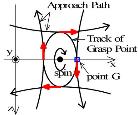
Fig.4 Grasp point velocity and approaching path
