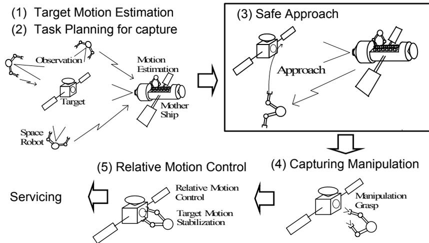
Fig. 1 Sequence of Satellite Capture
