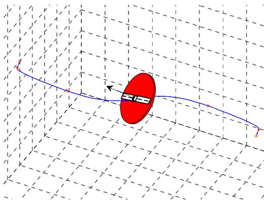
Fig. 12 Optimal Trajectories for Multiple Robots Approaching Simultaneously, x-z plane
