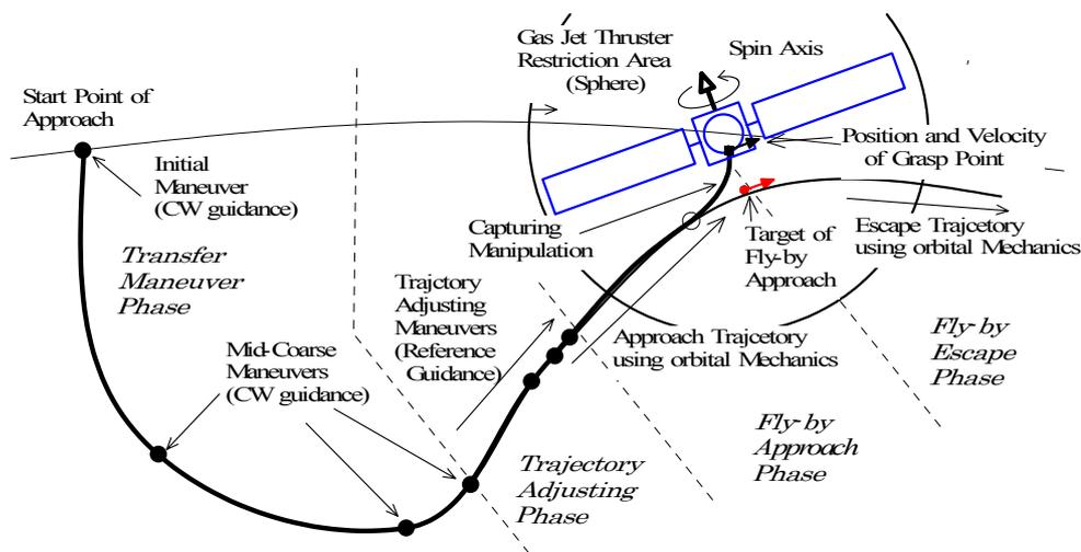
Fig. 2 Fly-by approach to target satellite
