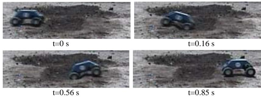
**Fig. 10.** Photo series of low-speed ditch traversal (1.4 m/s)
