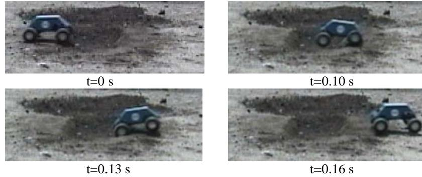
**Fig. 12.** Photo series of high-speed ditch traversal (7.4 m/s)
