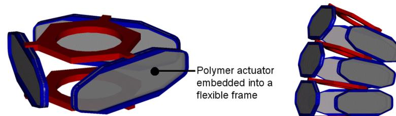
Figure 3 Polymer-actuated BRAID
