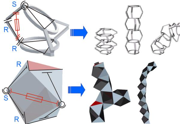
Figure 1 BRAID kinematics; top) RRS; bottom) RSR
