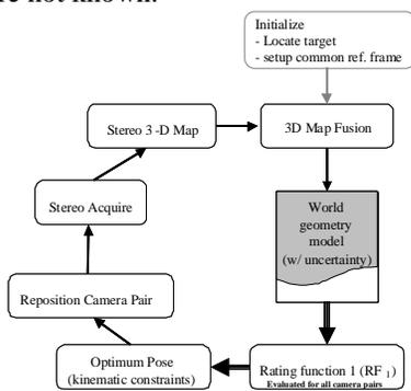
Figure 3: Outline of model building and placement algorithm
