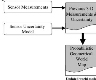
Figure 4: 3-D range measurement fusion with sensor uncertainty
