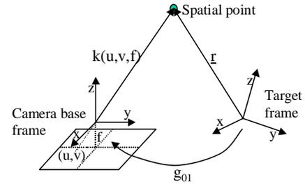
Figure 6: Relationship of camera and target frames
