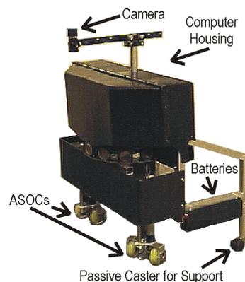
Figure 3: The SmartWalker with Its OMP
