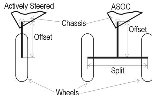
Figure 1: Actively Steered Caster and ASOC
