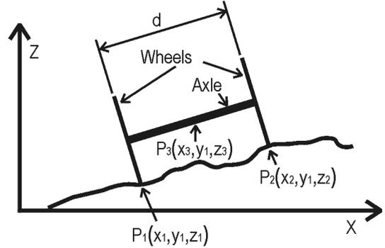
**Figure 6: ASOC on Uneven Terrain**
