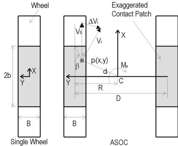
**Figure 11: Scrubbing Analysis for Notation for Single Wheel and ASOC Design**
