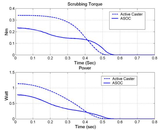
**Figure 13: Scrubbing Comparison of ASOC and Active Caster**
