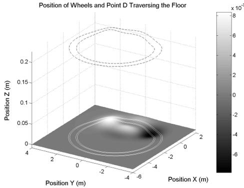
**Figure 10: Position of Wheels and Point D of the OMP Traversing Uneven Terrain**
