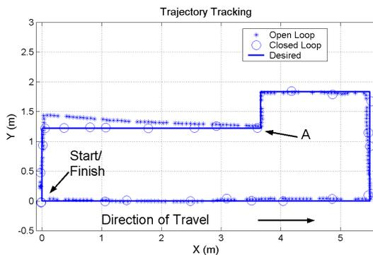
Figure 15: Open vs. Closed Loop Trajectory Tracking
