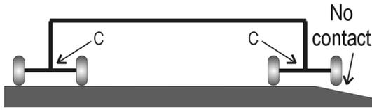
**Figure 4: Loss of Contact on an Uneven Floor**
