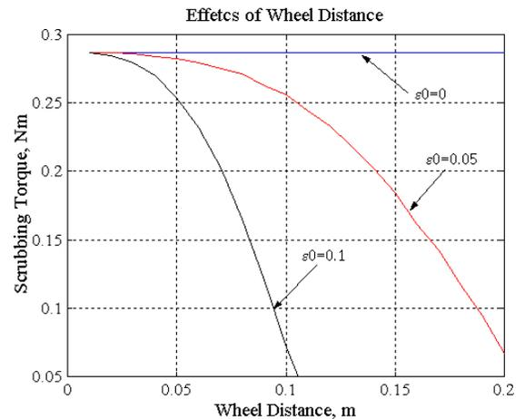
**Figure 14: Effect of Wheel Distance on Scrubbing Torque**
