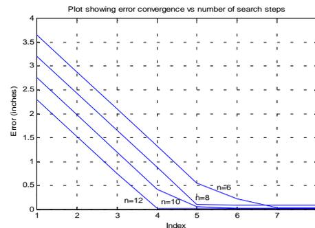
Figure 9: Results of combinatorial heuristic search algorithm for n-staged BRAID element (maximum allowable bit changes = 3)
