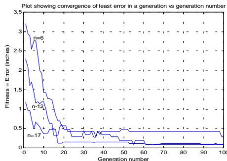
Figure 8: Results of genetic search algorithm for n-staged BRIAD element (population size = 30, probability of crossover = 0.6, probability of bit-wise mutation = 0.02) Figure 9 shows the performance of the combinatorial heuristic search algorithm, attempting to reach a desired position from an initial position. The algorithm was tested
