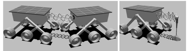
(a) mating two rovers (b) coring rock samples
