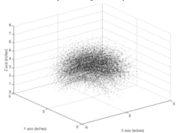
Figure 7: Workspace of 5 stage BRIAD element (BRAID element base center=origin)
