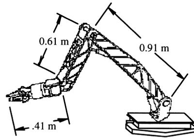
Fig. 10. Schilling Titan II mounted on a force/torque sensor.
