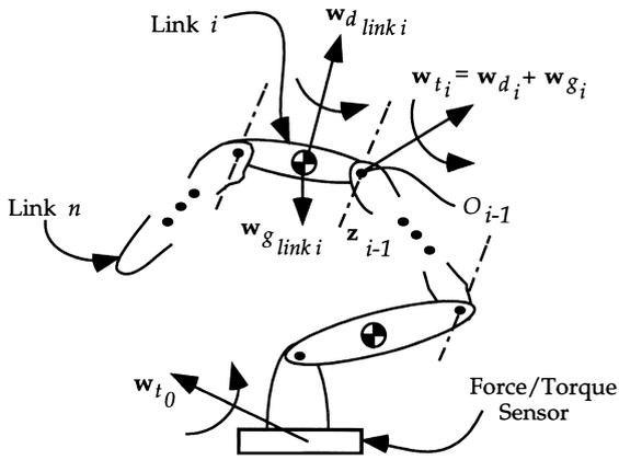
Fig. 1. Serial manipulator mounted on a base force/torque sensor.
