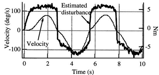
b. Estimated Disturbance Torque and Measured Joint Velocity
