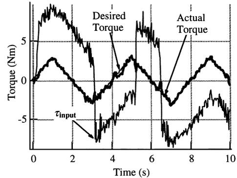
Fig. 6. Joint 1 torque control experimental results.
