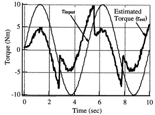
a. Torque Command and Base Sensor Measured Joint Torque
