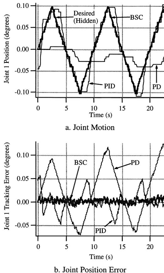
Fig. 8. Comparison of BSC and conventional control for a precise tracking task.
