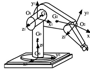
Fig. 3. Puma Denavit–Hartenberg link frames.
