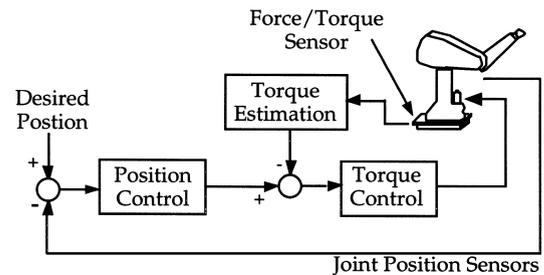
Fig. 7. BSC-based precision position control structure.
