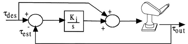
Fig. 5. Torque control block diagram.
