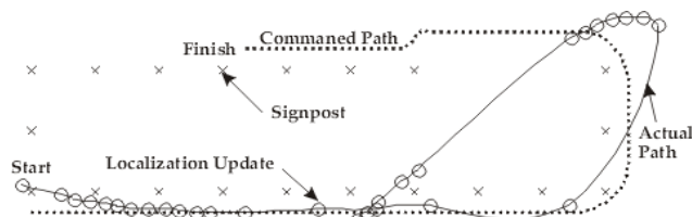
Figure 9. Experimental Tracking Performance without Localization Control.
