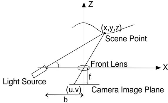
Figure 2: Project and Viewing Schematic
