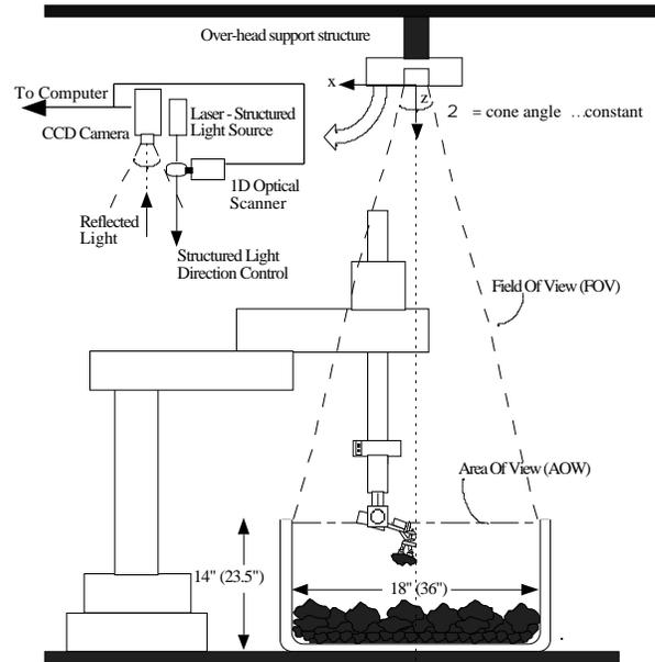
Figure 3: Overhead SGA vision system layout
