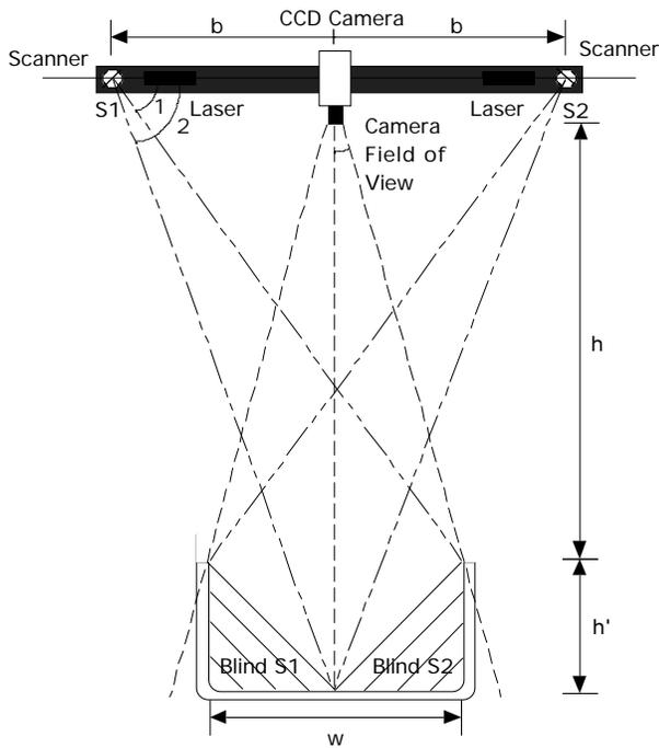
Figure 4: SGA design parameters
