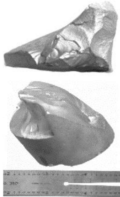
Figure 1: Typical polycrystalline silicon nuggets
