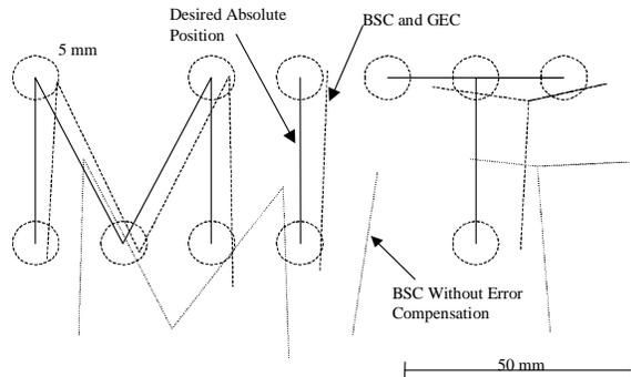
Figure 7 - Uncorrected and Corrected Accuracy
