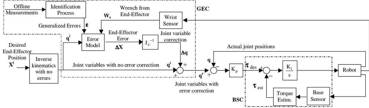
Figure 2 - Base Sensor Control and Error Compensation Scheme
