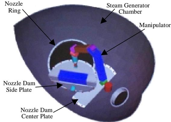
Figure 3 - Simulated Robotic Nozzle Dam Task
