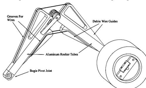
Figure 6: Reconfigurable Rocker Concept
