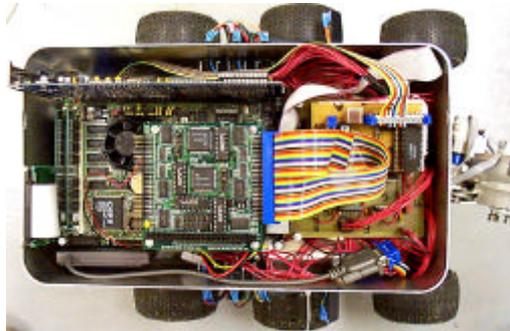
Figure 7: Rover Electronics Packaging
