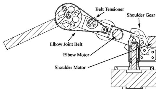
Figure 4: Three Degree-of-Freedom Manipulator
