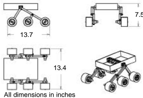
Figure 3: Experimental Rover Dimensions
