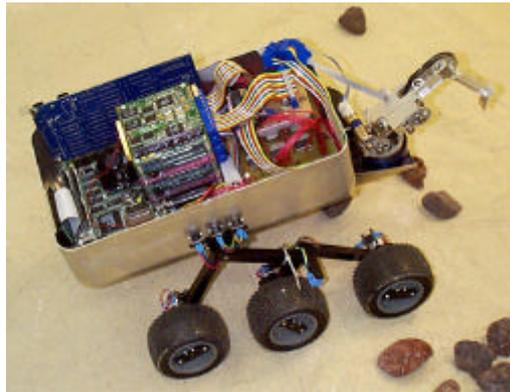
Figure 1: The Field and Space Robotics Laboratory (FSRL) Rover (without cover)
