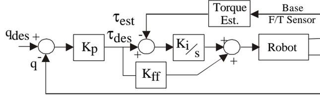
Figure 9: BSC Control Block Diagram
