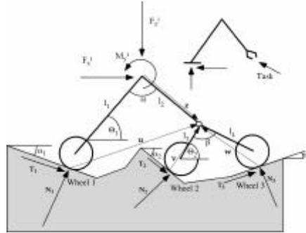
Figure 10: Traction Control Force Analysis
