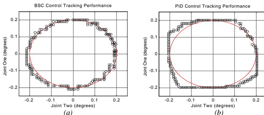
Figure 11: BSC Tracking Performance (Figure 11a) vs. PID (Figure 11b)
