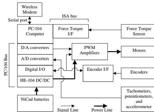
Figure 8: Electronic System Block Diagram
