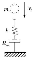
Figure 8. Dynamic impact model of ball and plate.
