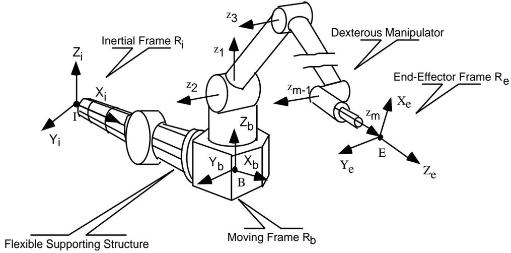
**Figure 2: Schematic of a general long reach manipulator system**
