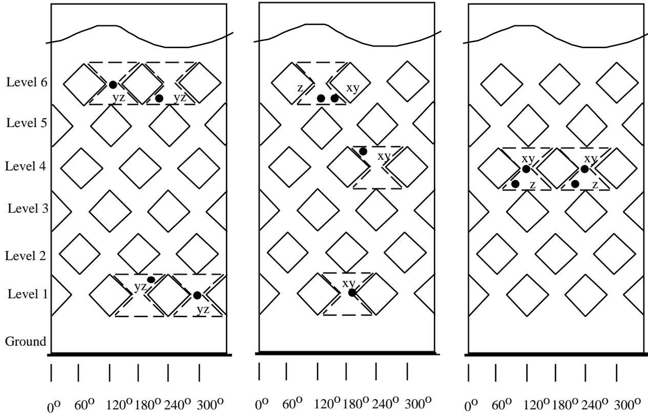
**Figure 9: Two "good" strain sensor locations and one "bad"**
