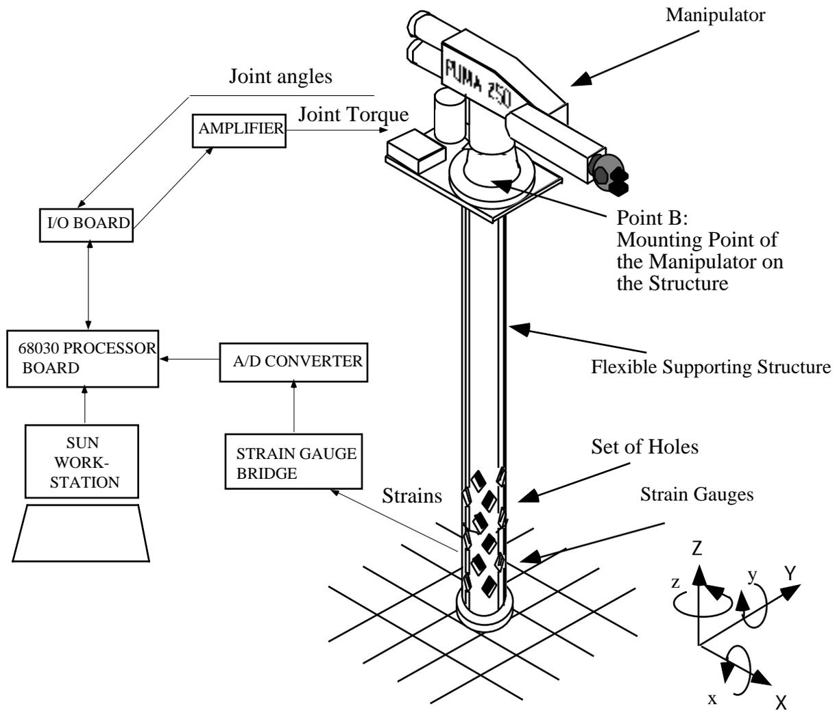
**Figure 7: Schematic of the MIT Spatial LRMS - Shaky II**
