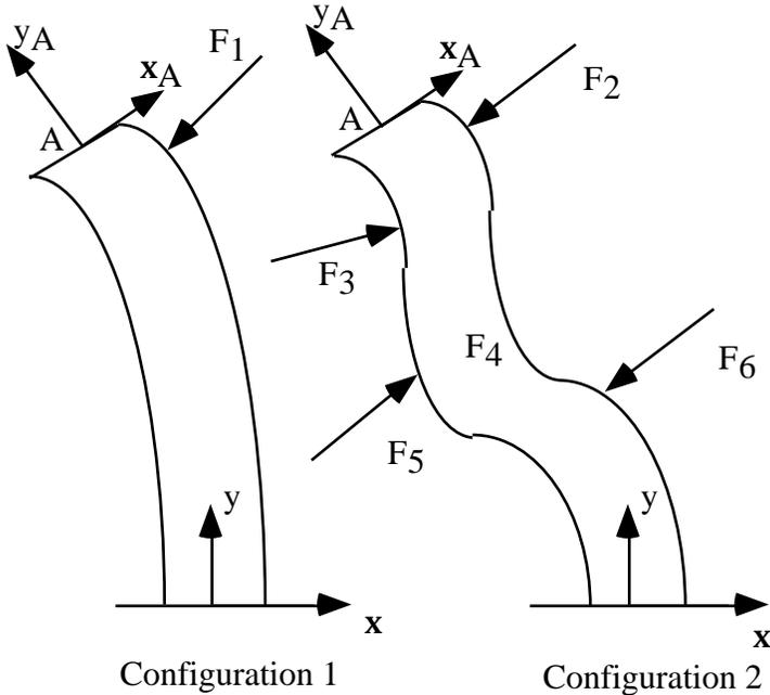
**Figure 4: Same displacement of point A with two different loading conditions**
