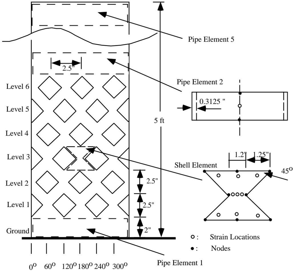
**Figure 8: Detailed schematic of the hole pattern**
