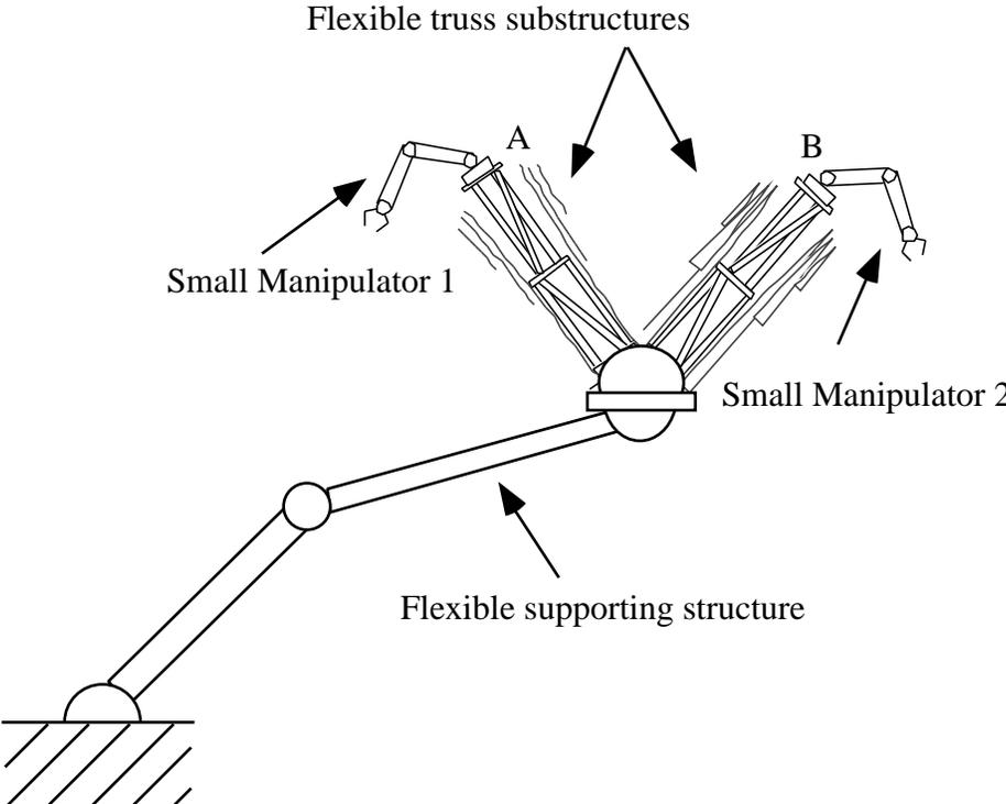
**Figure 3: Schematic of a complex two manipulator long reach system**
