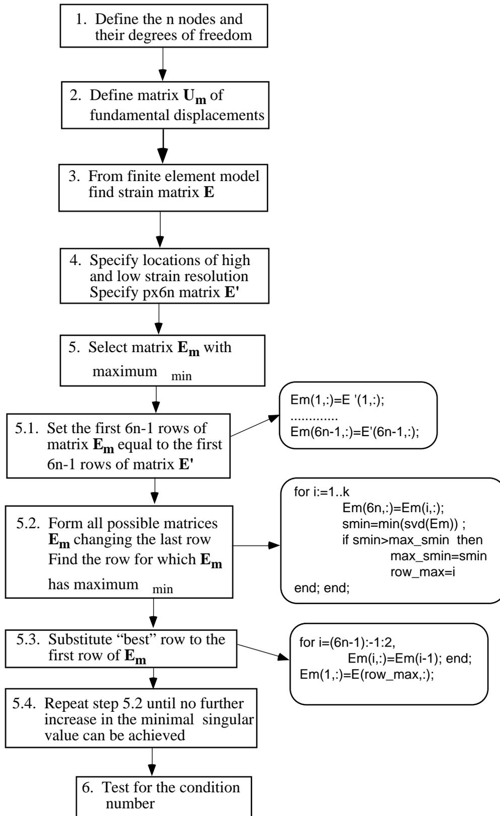
**Figure 5: Search algorithm for optimal strain placement**
