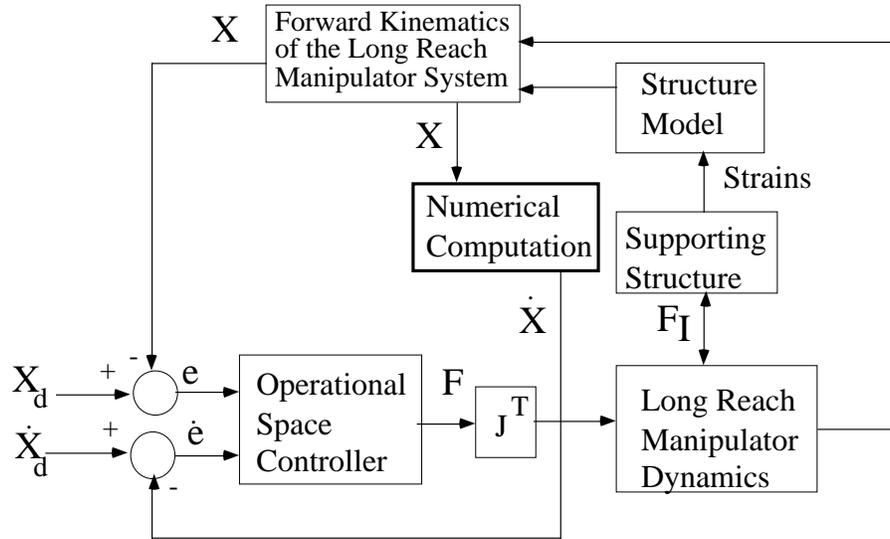
**Figure 6: Inferred End-Point Control algorithm for Long Reach Manipulators**
