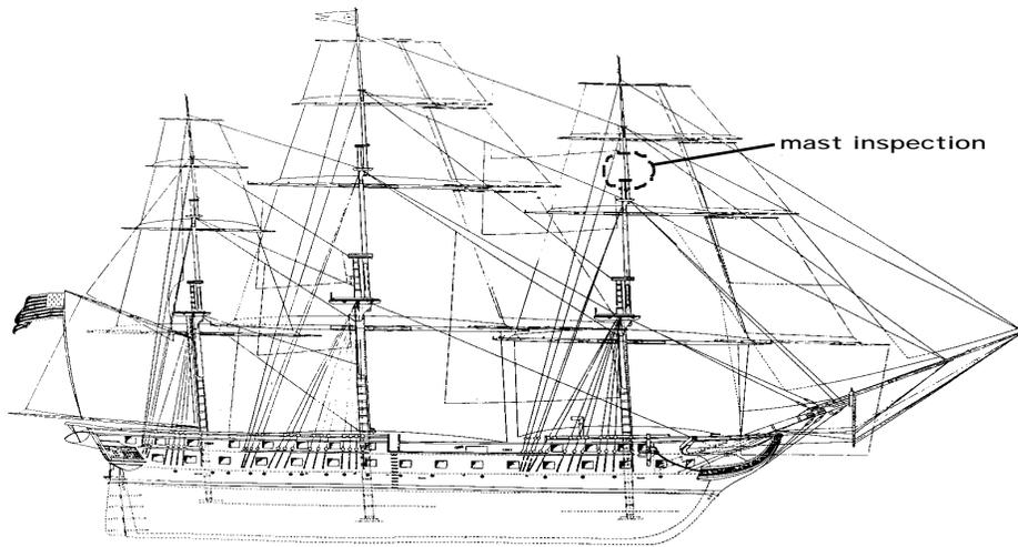
**Figure 6.** The complexity of the Constitution's rigging and height of her masts (220') make inspection difficult.
