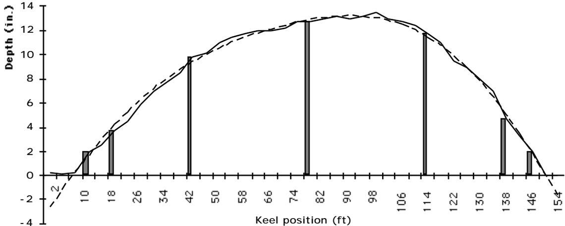
**Figure 3. Keel shape inferred from seven measurements. The bars are sensor readings, the solid line is diver-measured data, and the dashed line is the curve shape inferred from the sensors.**
