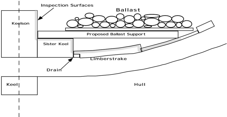
**Figure 4. Sub-ballast area. The area is only exposed during dry dock. An automated inspection system that can work underneath the ballast would be very useful.**
