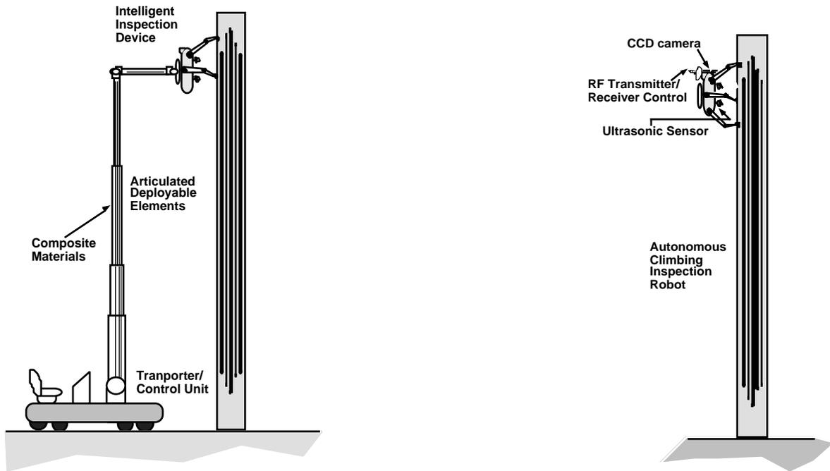
**Figure 7.** Two mast inspection robot concepts
