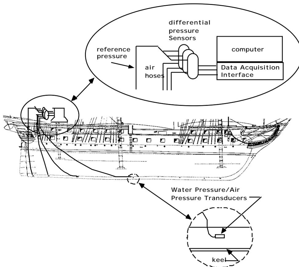
**Figure 2. The Hog measurement system overview. Sensors on the keel report pressure at specific locations, from which the computer calculates the keel shape.**
