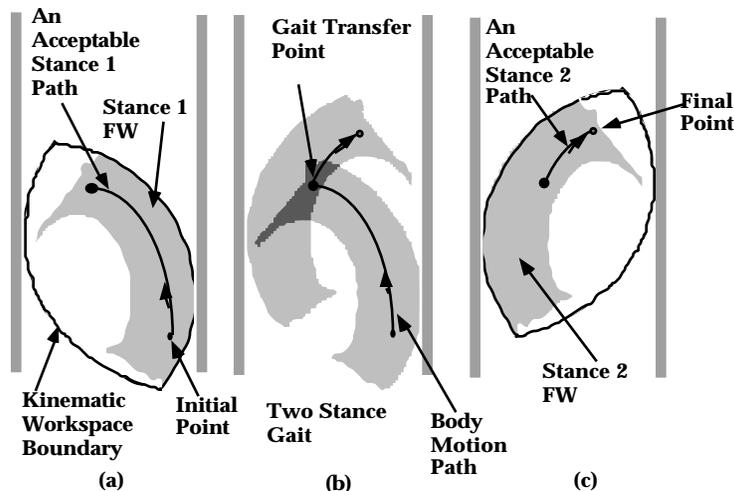
Figure 15. A gait generated using force-workspaces.
