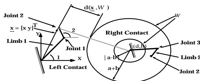
Figure 6. Finding the climbing robot's kinematic workspace.
