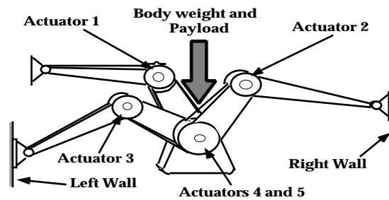
Figure 4. The Planar Climbing Robot Concept
