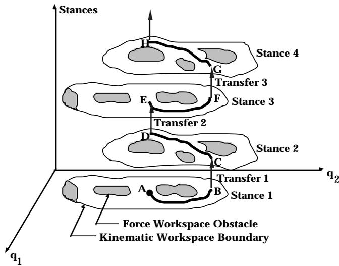
**Figure 14. Transferring between force-workspaces when choosing new contacts.**
