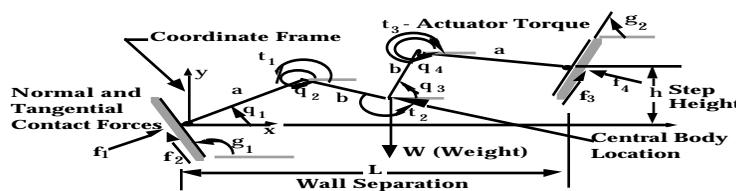
Figure 5. Kinematic Schematic of the Climbing Robot
