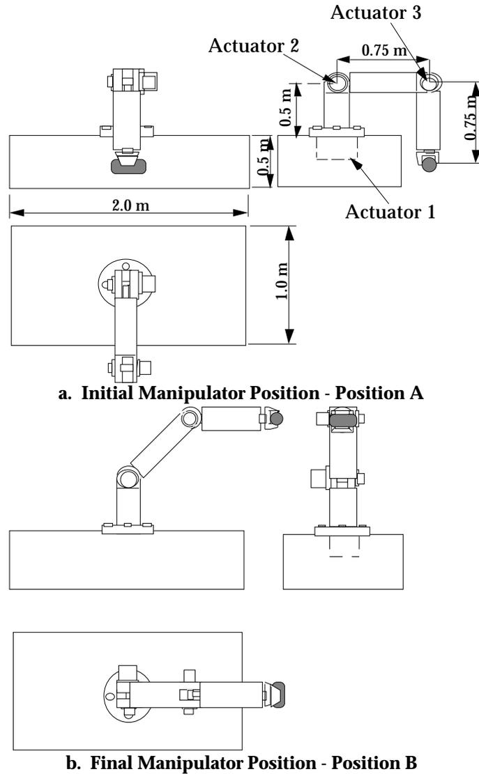
**Figure 5. Initial and Final Manipulator Positions**
