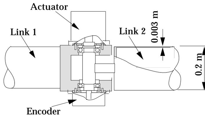
**Figure 4. Model of Manipulator Joint 2**
