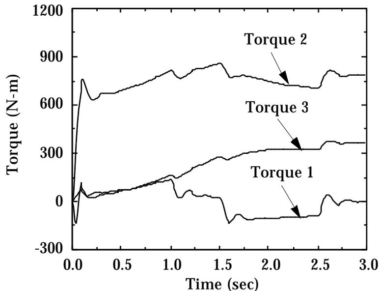
**Figure 9. Joint Torques - Flexible Links, Locked Suspension System**
