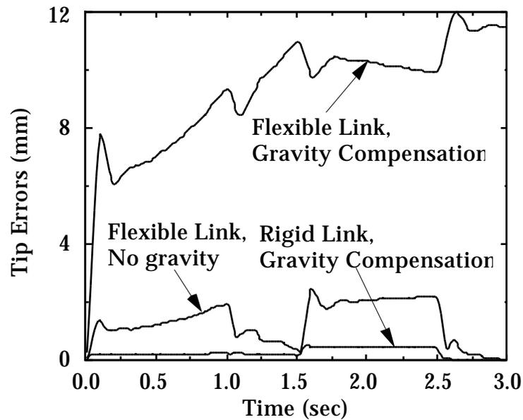
**Figure 7. Tip Errors for Locked Suspension System - Rigid and Flexible Links**
