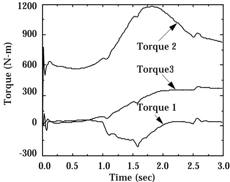
**Figure 12. Joint Torques - Flexible links with Flexible Suspension**
