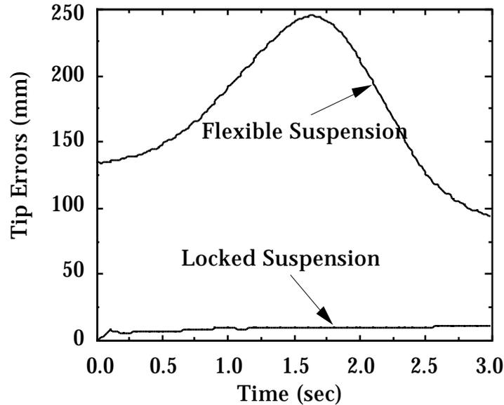
**Figure 10. Tip Errors for Flexible Suspension System - Flexible Links**
