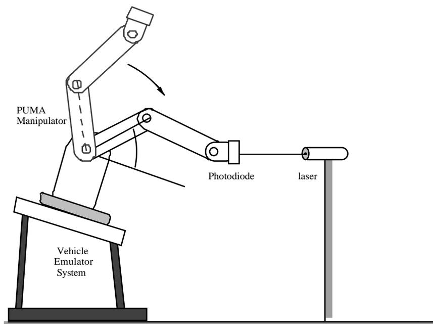
Figure 3. Sketch of Manipulator under Endpoint Feedback Control on a Compliant Base
