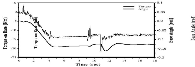
Figure 6. Endpoint Servoing of Manipulator on A Soft Compliant Base
