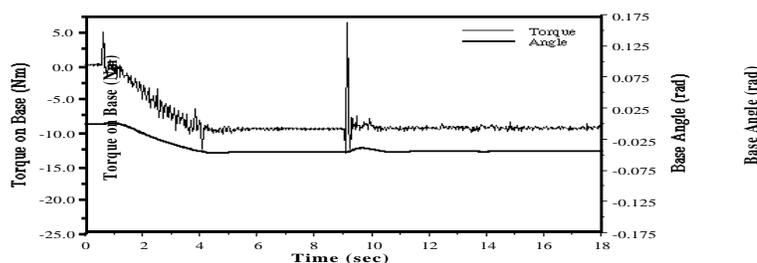
Figure 5. Endpoint Servoing of Manipulator on A Stiff Compliant Base
