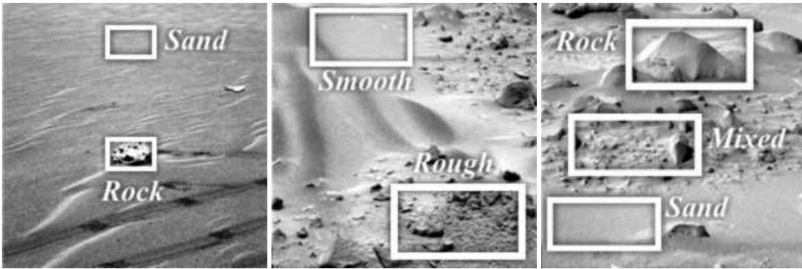
**Figure 2:** Class distinctions: color- and geometry based classes (left), texture-based classes (middle), fusion classes (right)
