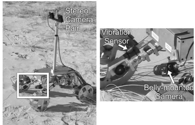
**Figure 6:** TORTOISE experimental rover (left), local sensing suite (right)
