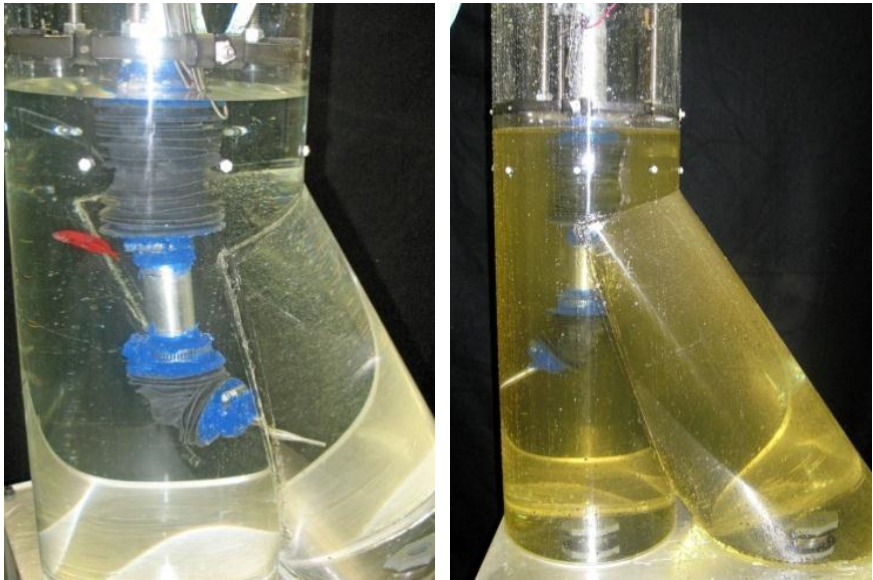
Fig. 8. Experimental robot submersed in water (left) and in a viscous sucrose solution (right).
