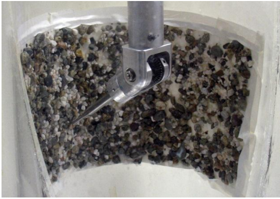
Fig. 7. The surface of a cylinder is covered with gravel, and the ability of the robot to determine the approximating cylinder is evaluated.
