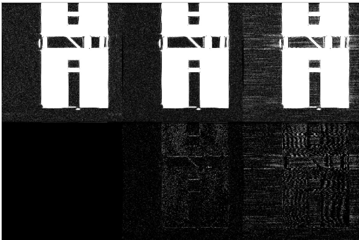
Fig. 14. Susceptibility artifact assessment. **Top:** from left to right: baseline, DEAs actuating with device in use-case location, DEAs actuating with device touching phantom. **Bottom:** the baseline image subtracted from the top images. No distortion to the left side of the phantom, which is in proximity to the device, is noted. The horizontal lines in the top right image are due to electromagnetic interference, not susceptibility.
