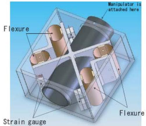
**Figure 9. Force/torque sensor design**
