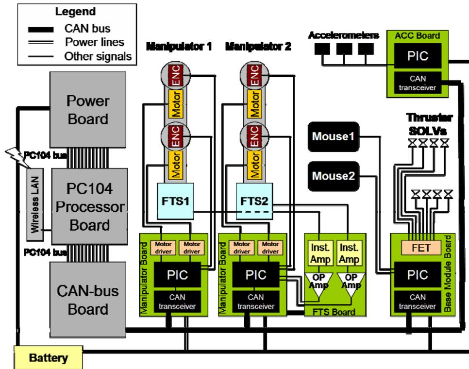
Figure 10. Electronics Diagram
