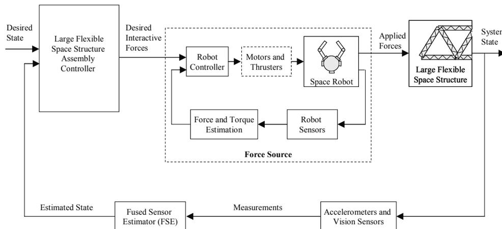
**Figure 3. Block diagram for the decoupled controller**
