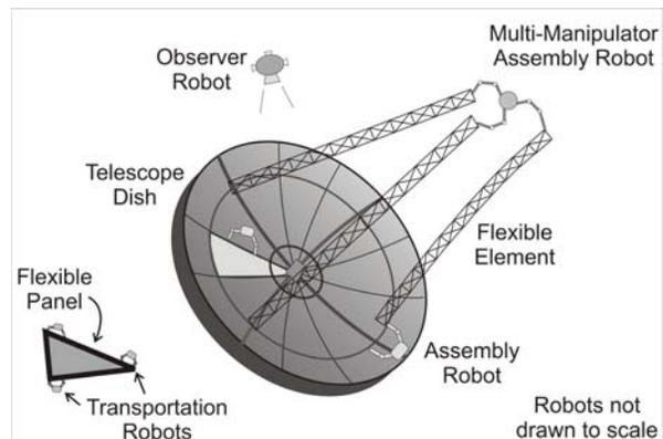
**Figure 1. On-orbit construction of a flexible telescope by teams of space robots**
