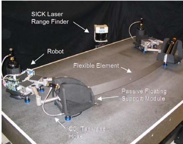
**Figure 2. The MIT experimental testbed**
