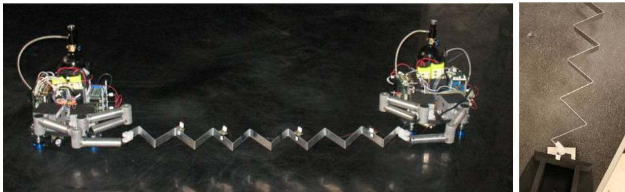
**Figure 12. Zig-zag flexible element prototype**
