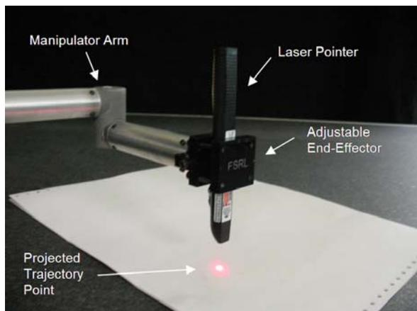
**Figure 8. End-effector holding laser pointer**
