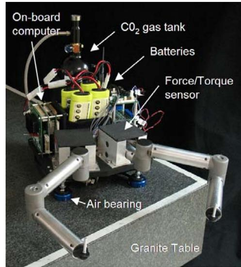
Figure 5. Experimental space robot
