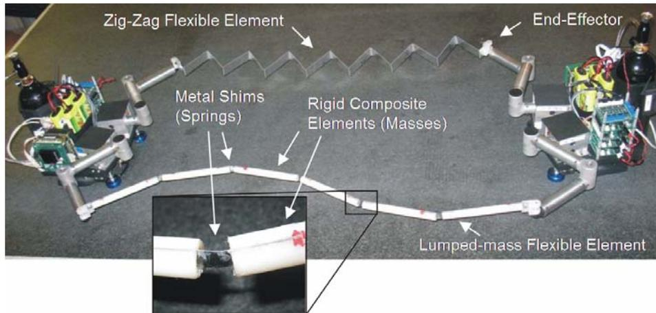
**Figure 13. An overhead view of two robots manipulating lumped-mass and zig-zag beam**
