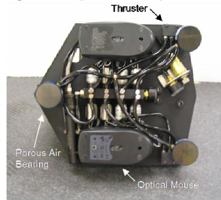
Figure 6. Underside of experimental robot
