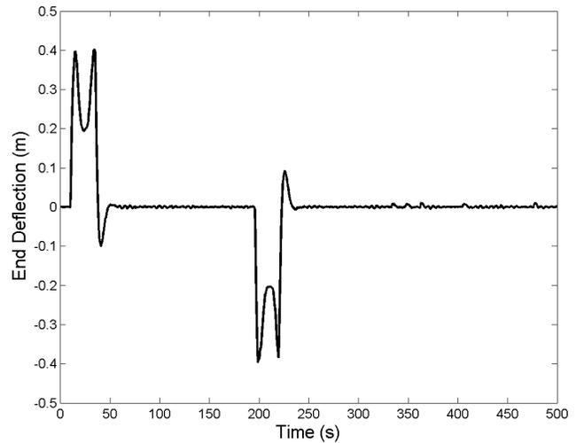
Fig. 6 End deflection of beam during maneuver – with vibration measurements.
