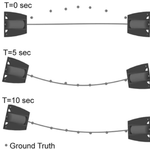
Fig. 20. Estimate from 3 structure-mounted accelerometers and 9-Hz vision data.
