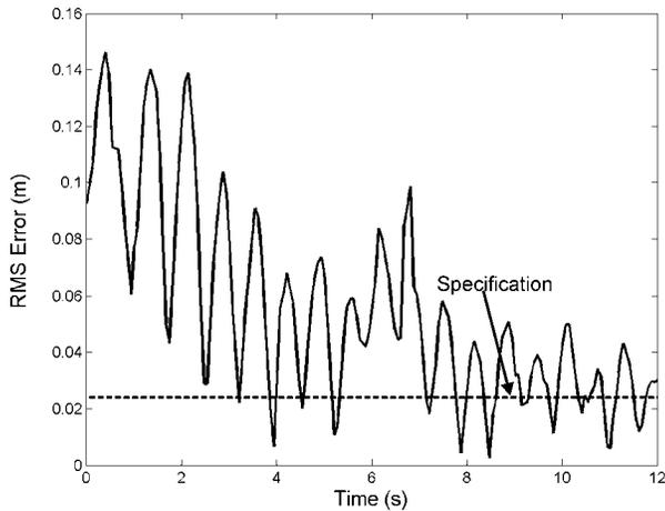
Fig. 17. RMS error of an estimate using 3 accelerometers.
