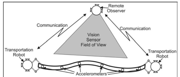
Fig. 2. Maneuvering of large flexible structure by cooperative robots.
