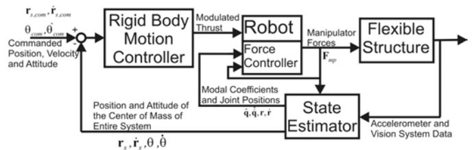
Fig. 3. Control architecture [3].
