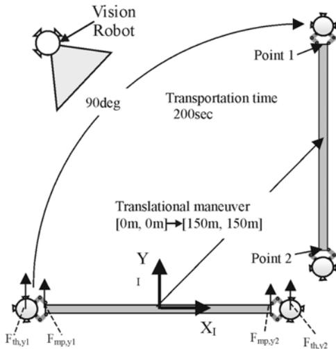
Fig. 4. Transportation maneuver using a team of robots.
