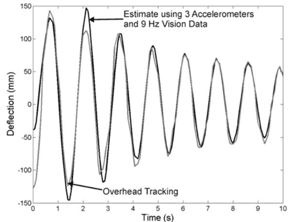
Fig. 19. Tracking of a point 8 cm along the structure using an estimate from 3 accelerometers and 9 Hz vision data.
