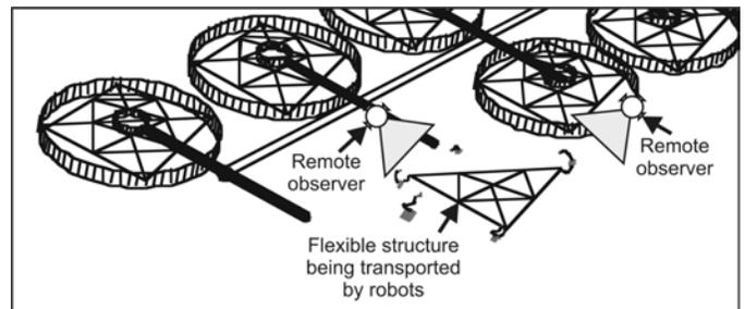
Fig 1. In-orbit construction of LSS by cooperative robots.
