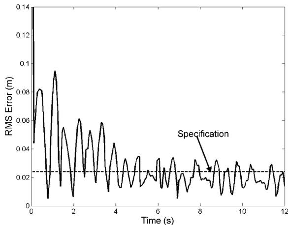
Fig. 13. RMS error of an estimate using 9 Hz vision data.
