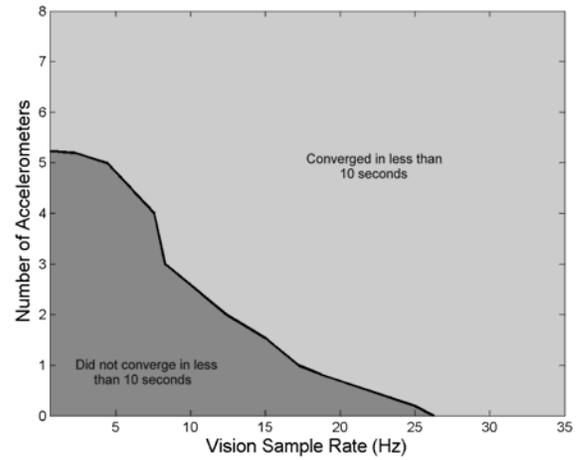
Fig. 18. Sensor configurations, experimental results.
