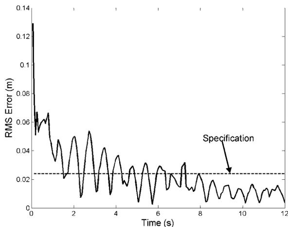
Fig. 21. RMS error of an estimate using 3 accelerometers and 9 Hz vision data.
