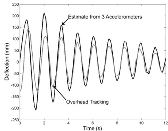
Fig. 15. Tracking of a point 8 cm along the structure using an estimate from 3 accelerometers.
