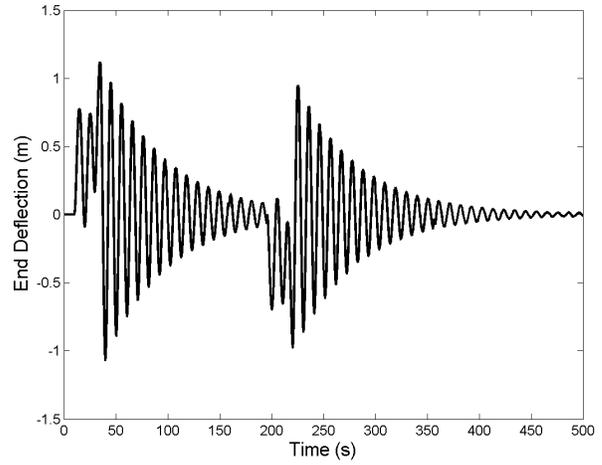
Fig. 5. End deflection of beam during maneuver - without vibration measurements.
