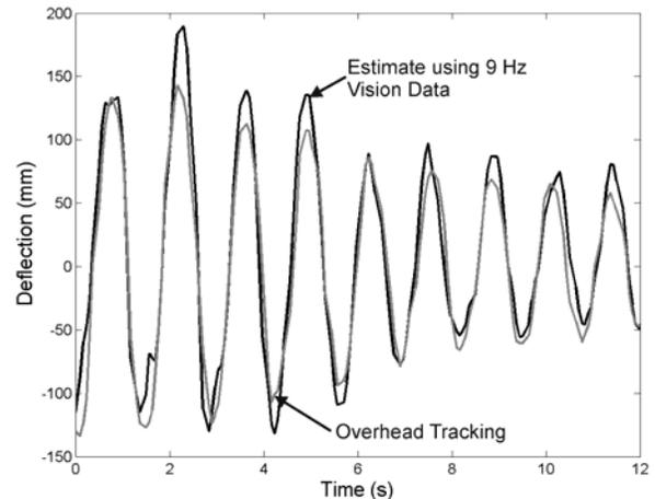
Fig. 11. Deflection of a point 8 cm along the structure using an estimate from 9-Hz vision data.
