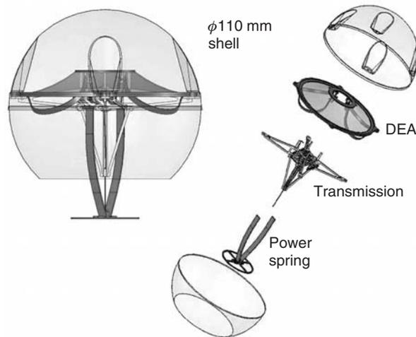
**Figure 26.10** Microbot mobility concept.
