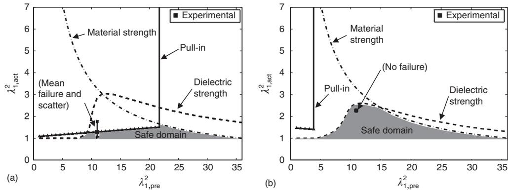
**Figure 26.5** Failure analytical predictions for (a) low stretch rate ( $\dot{\lambda}_{uni} = 3.3 \times 10^{-4} \text{ s}^{-1}$ ) and (b) high stretch rate ( $\dot{\lambda}_{uni} = 0.0945$ ) with loading stress [15].
