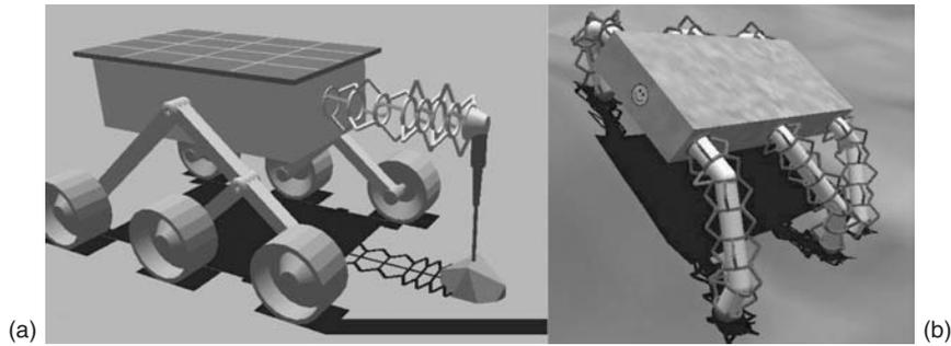
**Figure 26.2** Example of binary robotic applications: (a) manipulator on a conventional rover and (b) legs of a walking robot.
