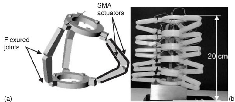
**Figure 26.4** The MIT SMA powered binary manipulator [18]: (a) single-stage and (b) five-stage devices.
