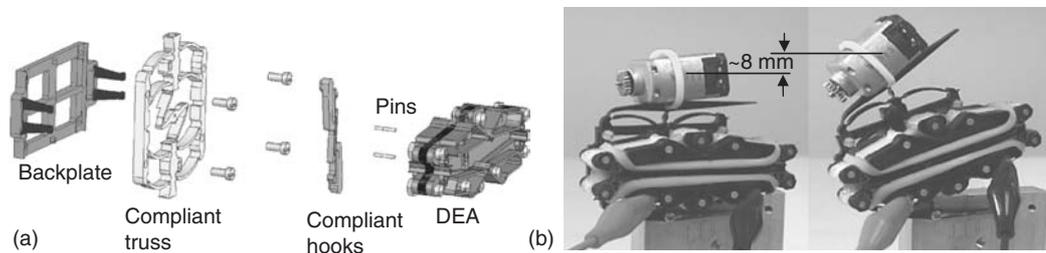
Figure 26.8 Bi-stable module using a single actuator: (a) exploded view and (b) prototype.
