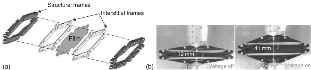
**Figure 26.3** DEA with linear extensions greater than 100%: (a) exploded view and (b) prototype.
