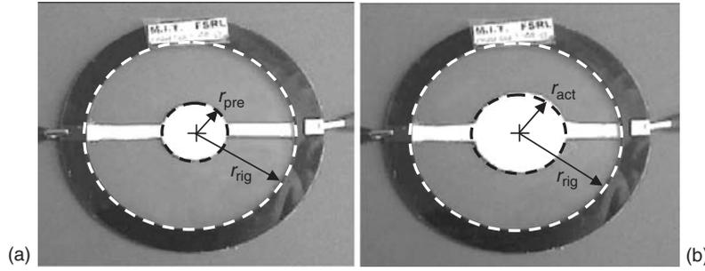
Figure 26.12 Expanding circle: (a) pre-stretched ( $V = 0$  kV) and (b) actuated ( $V = 10$  kV).
