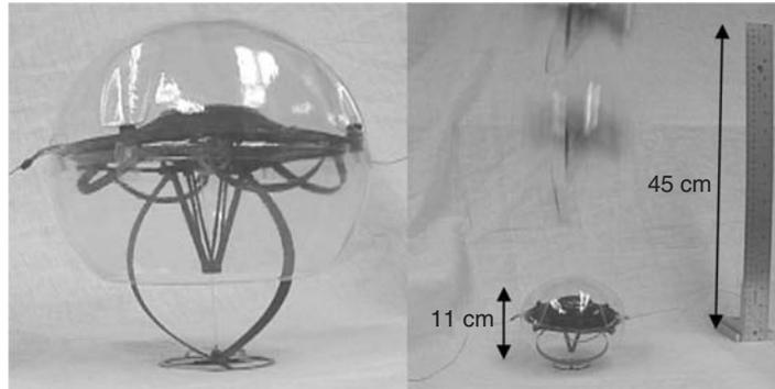
Figure 26.11 Microbot prototype performing hops of 60 cm.
