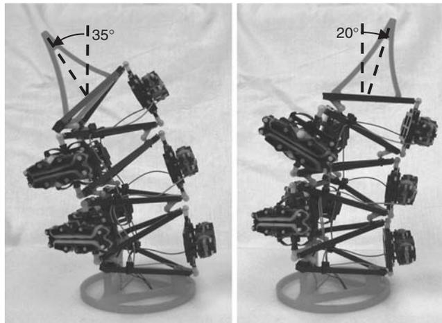
**Figure 26.6** A 7-DOF binary manipulator prototype.
