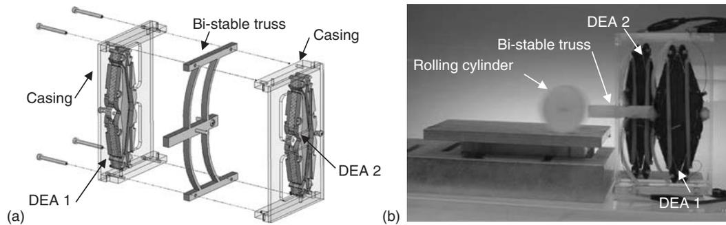
Figure 26.7 Antagonistic bi-stable module: (a) exploded view and (b) prototype.
