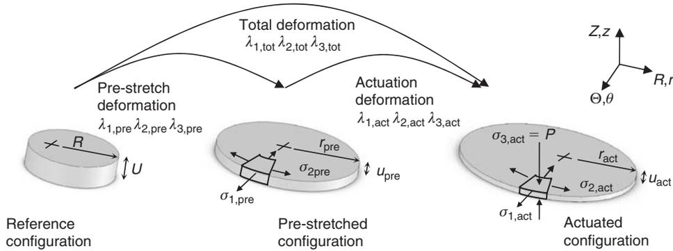
Figure 26.13 The deformations and stresses of the active region.
