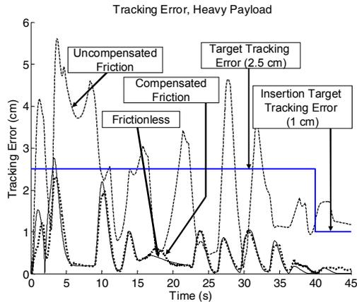
Fig. 7 Heavy payload representative task tracking error
