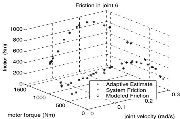
Fig. 11. Comparison of the adaptive friction estimates with the system friction and curve-fit model friction.
