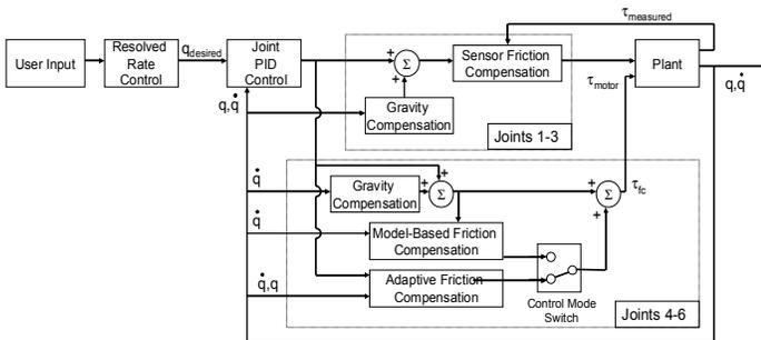
Fig. 5 Block diagram of control architecture
