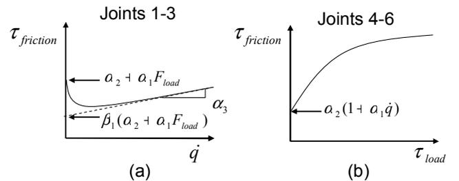
Fig. 2 (a) Friction models for joints 1-3 as a function of velocity at constant load, and (b) joints 4-6 as a function of motor load at constant velocity
