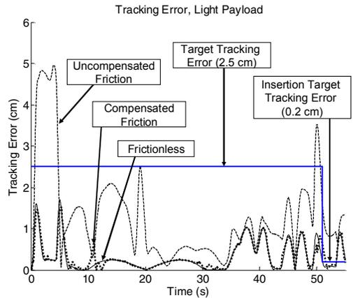
Fig. 8 Light payload representative task tracking error
