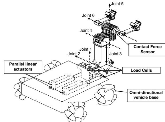
Fig. 1 Manipulator joint definitions (courtesy of Foster Miller Inc.)
