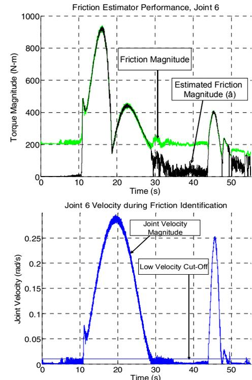
Fig. 10. Adaptive friction estimator performance for joint 6 during the light payload task.
