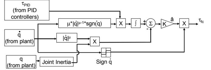
Fig. 6. Block diagram of adaptive compensation algorithm
