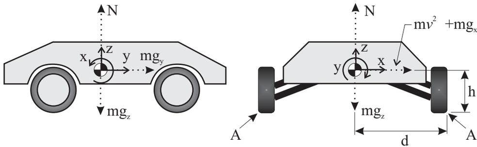
Figure 3: Free body diagram of a UGV.
