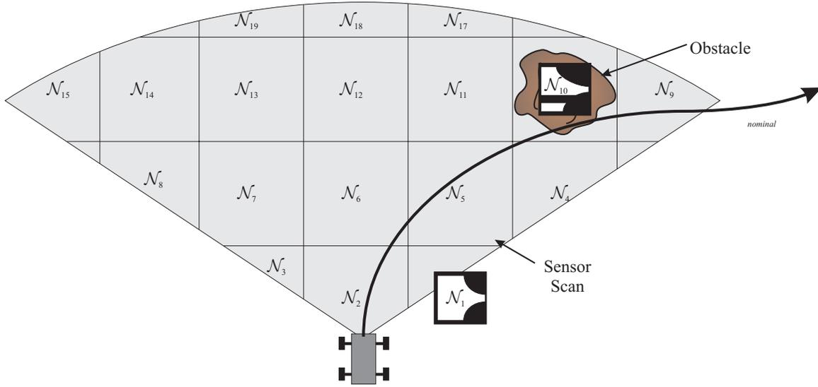
Figure 9: Admissible Trajectory Spaces defined with hazard present.
