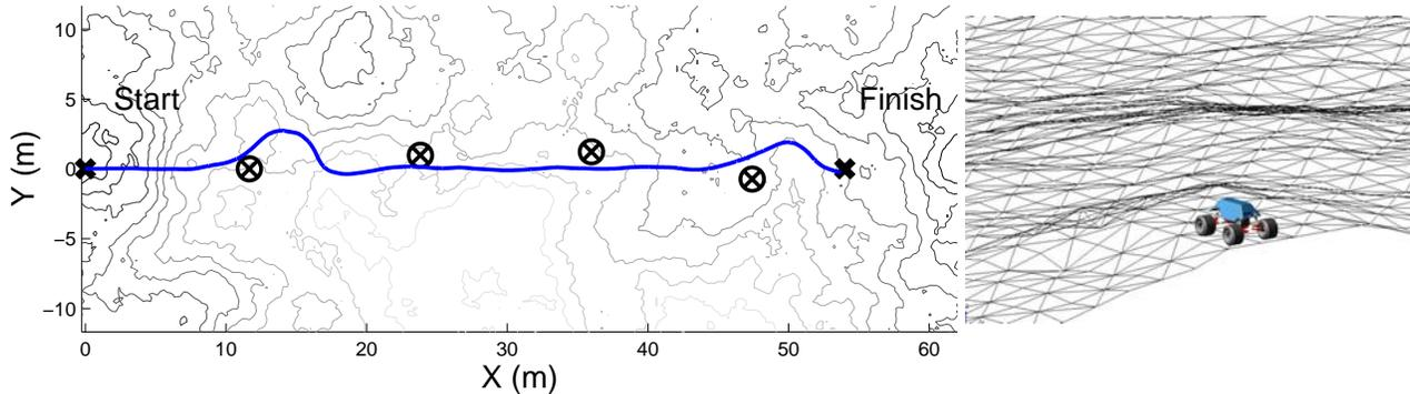
Figure 12: Hazard avoidance simulation results (left). A circled X indicates a hazard location. Hazard sizes are seven wheel diameters (1.45 m) wide. Terrain used in the simulation (right).
