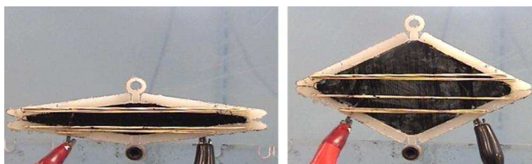
FIGURE 9. Experimental Dielectric Elastomer Actuator with 200 Percent Strain.
