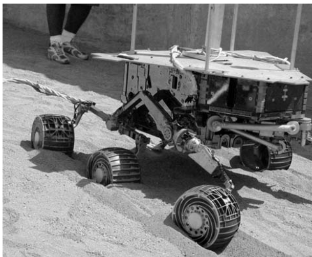
Fig. 1 Significant wheel sinkage on mockup of Spirit rover at NASA Jet Propulsion Laboratory (NASA/JPL Image)
