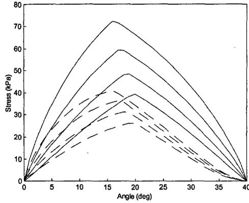
**Figure 2:** Normal stress (solid) and shear stress (dashed) distribution for varying slip and sinkage
