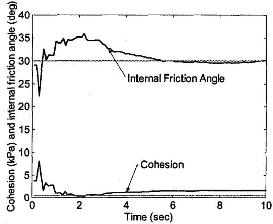
Figure 3: Simulated comparison of estimated cohesion (black) and internal friction angle (black) estimation to true values (gray)
