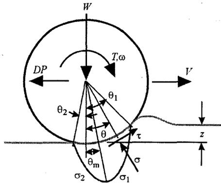
Figure 1: Free-body diagram of rigid wheel on deformable terrain
