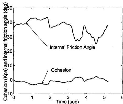
Figure 6: Experimental results of cohesion and internal friction angle estimation
