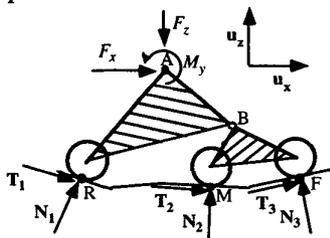
Figure 4. Planar rover force analysis
