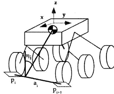
Figure 3. Rover stability criterion
