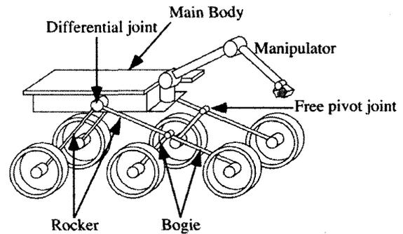
Figure 1. A rocker-bogie class rover
